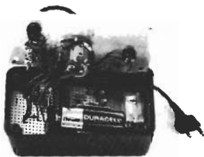
FIG. 2—THE PROJECT IS HOUSED in a small project box with an aluminum front panel. Note the lead to the recorder at the right; it was taken from a defective microphone (see text).
