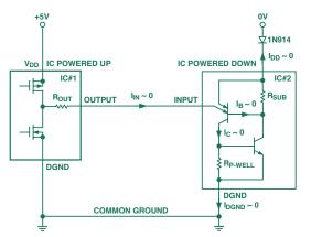
Figure 4. Addition of a diode in series with  $V_{\text{DD}}$  prevents SCR triggering.
