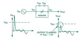
Figure 8. Channel protector clamps overvoltages to within power supply rail voltage and protects sensitive components.
