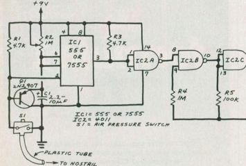
Fig. 6. This circuit monitors respiration and emits a warning tone when time between breaths exceeds a predetermined interval.
