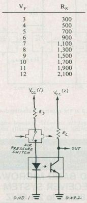
Fig. 3. The air pressure switch can be isolated from the controlled circuit by an opotoisolator.
