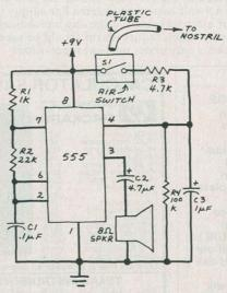
Fig. 5. Respiration indicator provides audible signal.
