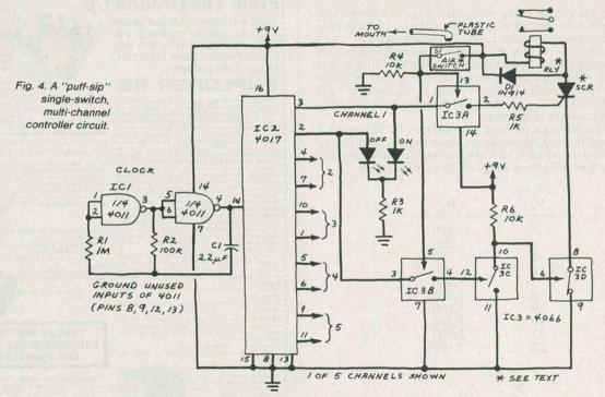
be turned on by puffing or sipping on the plastic tube connected to the circuit's single PSF 100A air switch. Depending upon the value of CI, the operator has up to a second to operate the air switch. If more time is required, the value of CI
