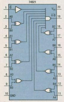
Fig. 3. The 74521 is technically known as an 8-bit identity comparator. Its output will go low provided each of its A inputs matches its corresponding B inputs and the enable input (G) is low.
