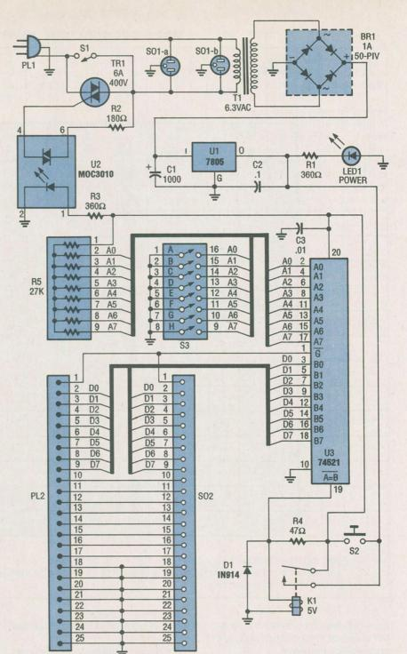
Fig. 4. At long last, here is the schematic diagram for the Kill Switch. Note how the 74521 is connected directly to the data lines.
