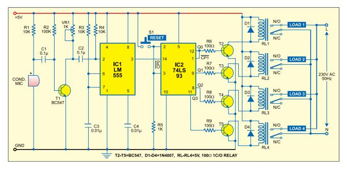
used in this circuit, which you can keep by the bedside. You can switch on/off up to four different electrical equipment (TV, fan, light, etc) in 16 different ways.
