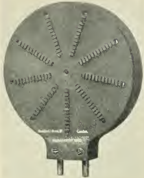
The Gambrell Inductance, a type having very low self capacity.
