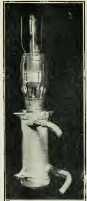
Fig. 109. The valve anode inserted in a water circulated cooling jacket.
