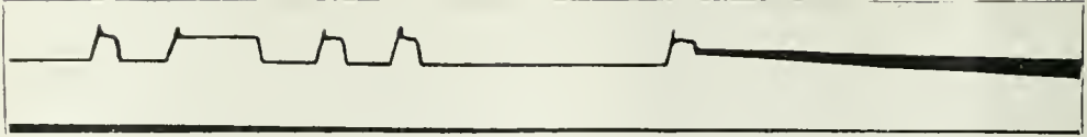
FIG 12.—THE SIPHON PEN, ON THE RIGHT, TRACING OUT IN MORSE ALPHABET, THE FIRST WORD—"LE"—OF COMMANDANT FERRIÉ'S MESSAGE
