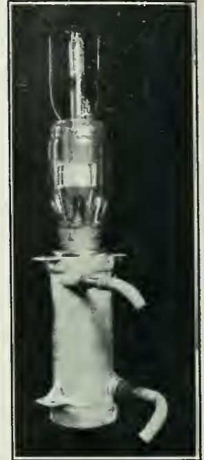
ABOVE: Valve inserted in water circulated cooling jacket.
