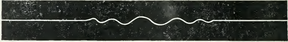
Fig. 2. The two components of a mechanical lantern slide for demonstrating wave motion. The white lines represent the transparent portions. The grid and wave line stand face to face in
