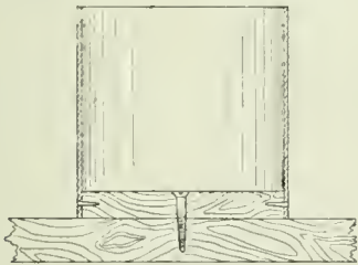
Fig. 7. Method of attaching the fixed coil to the base.
