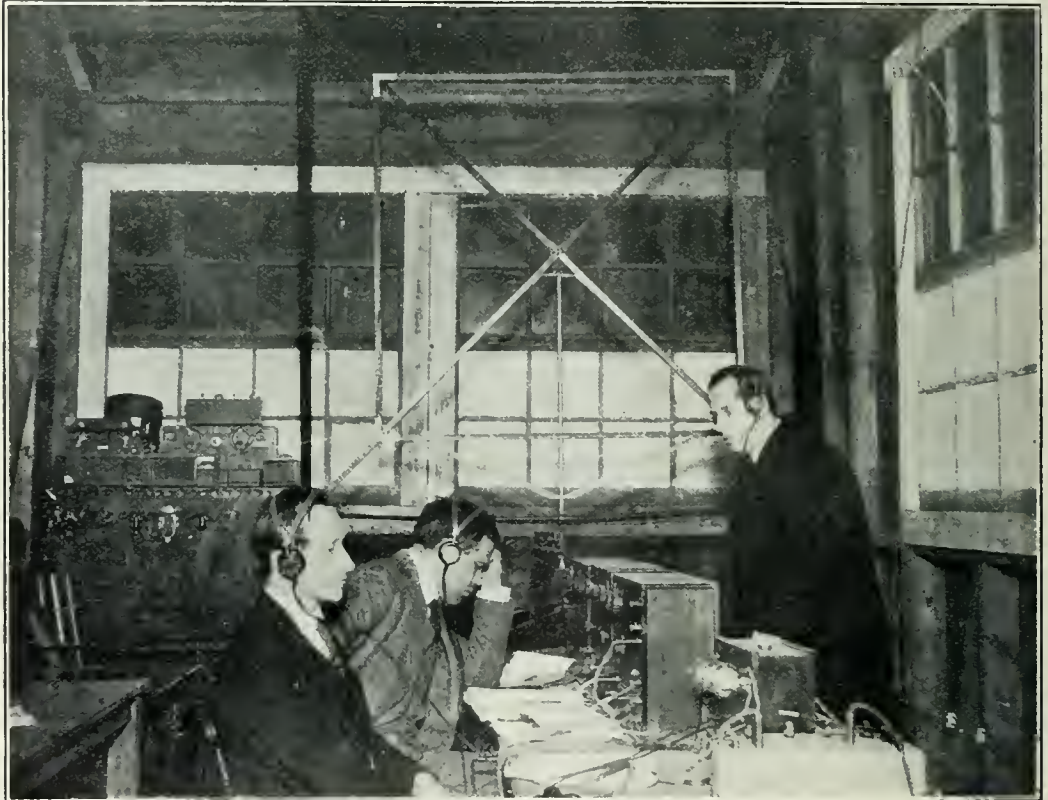
The frame aerial, having 6 ft. sides, and the apparatus with which the signals were received. Mr. Freiss, the Research Engineer, is in the centre.
