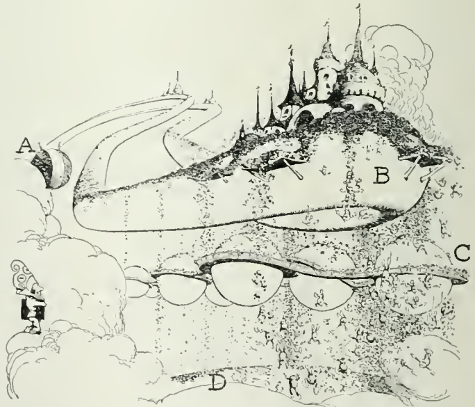
Fig. 12. The upper object represents the heated filament, projecting electrons, depicted as little imps, towards the plate and impeded in their progress by the grid.
