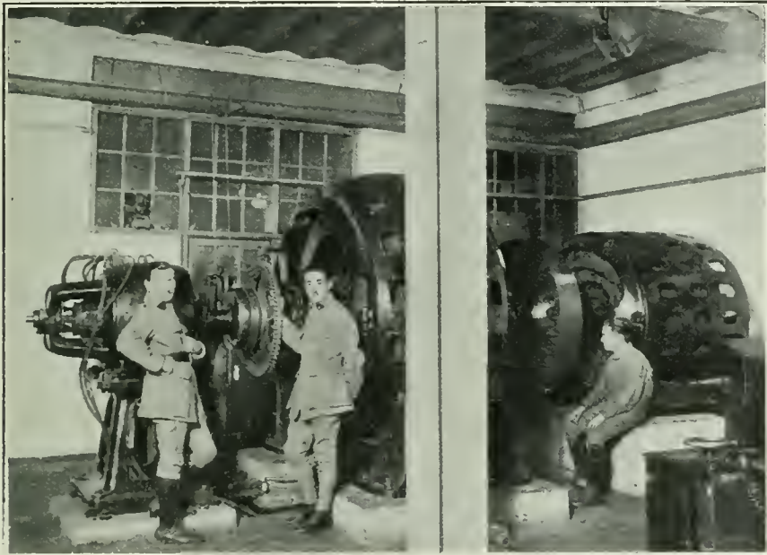
Fig. 5. Asynchronous 3-phase motor coupled to 500-kW. Generator which feeds the Spark Transmitter.
