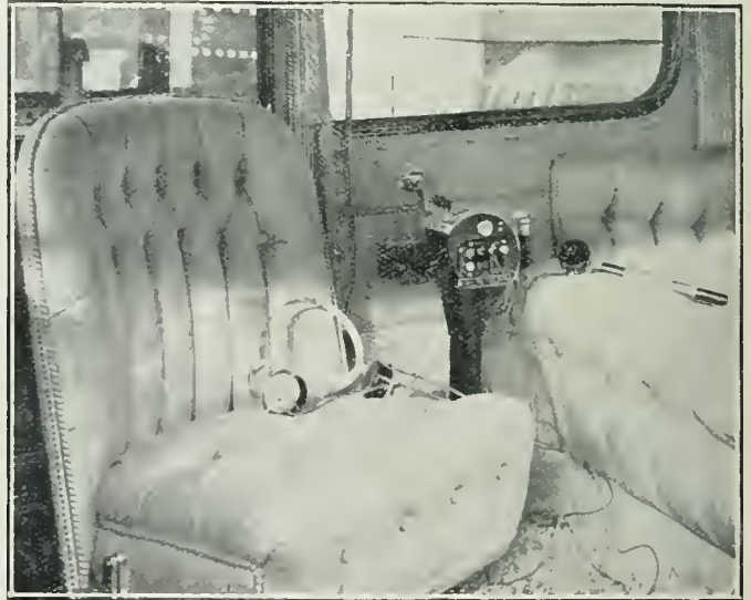
The Receiving Set, which was connected to a frame aerial carried on the roof of the car.
