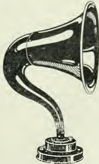
Fig. 82. Loud speaking Telephone of S. G. Brown.
