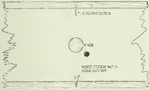
Fig. 6. Method of fixing back so as to allow easy removal.
