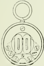
Fig. 80. Watch form of Magneto-Telephone receiver with the diaphragm removed to show the magnet and the coils.
