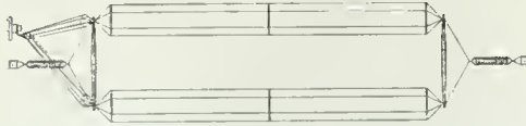
The figure gives an outline of a cage, inverted L type aerial. Those who expect to generate up to about 100 watts in the aerial circuit would find a single cage satisfactory.
