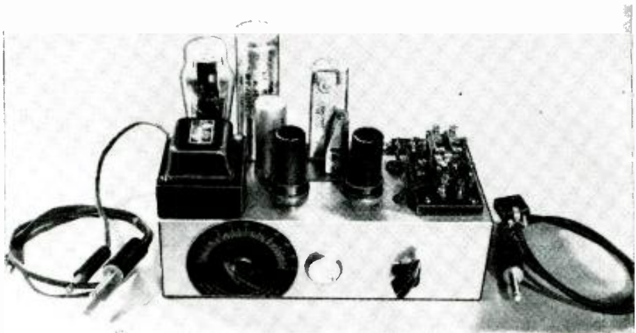
Fig. 2—This 3-tube relay unit operates recorder when a signal is transmitted or received.
