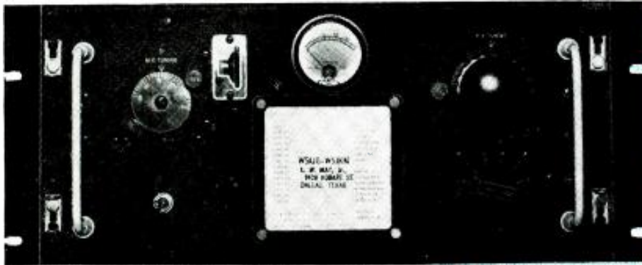
Metal extensions allow placing panel in standard rack.
