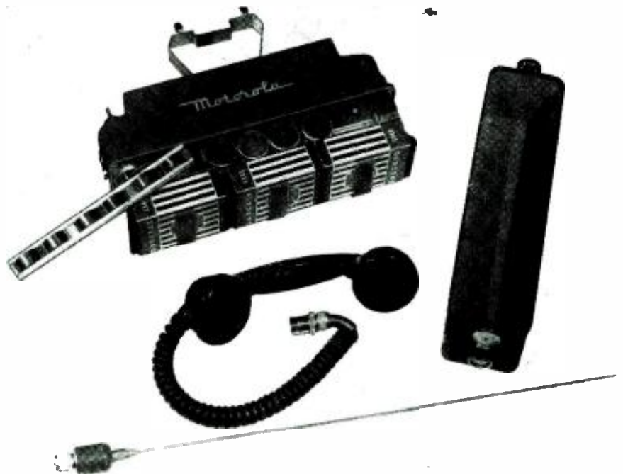
This is the portable radioset. The antenna, handset and bottom cover have been removed.
