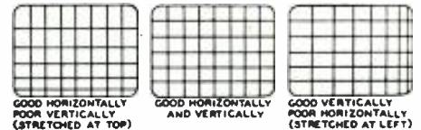
Fig. 3—Grid pattern is good linearity check.
