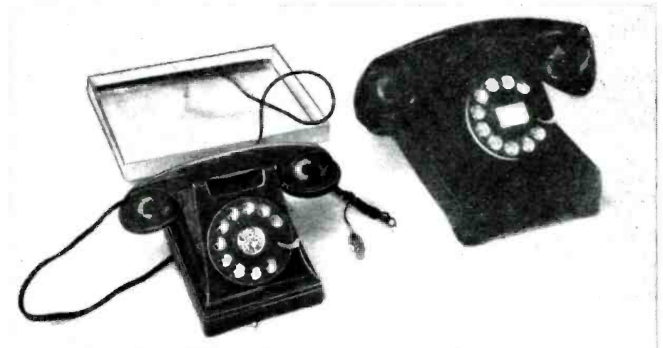
Fig. 3—Toy radio at left is tuned by turning the "telephone" dial. Standard phone at right.
