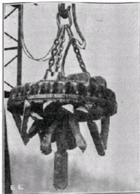
Modern Type Electro-Magnet Lifting Pig Iron from Freight Car.
