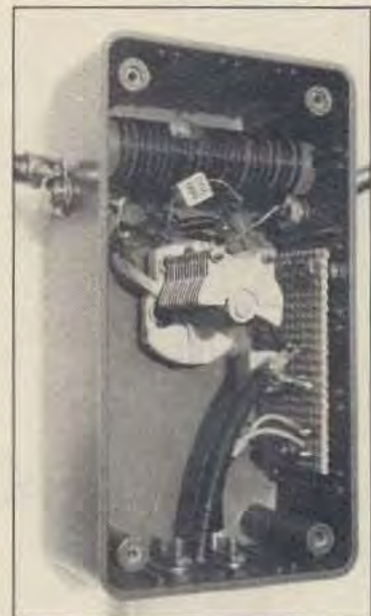
Photo B. Inside the HF Homer enclosure. Stator terminals of C1 are clipped off to make it fit in the box.
