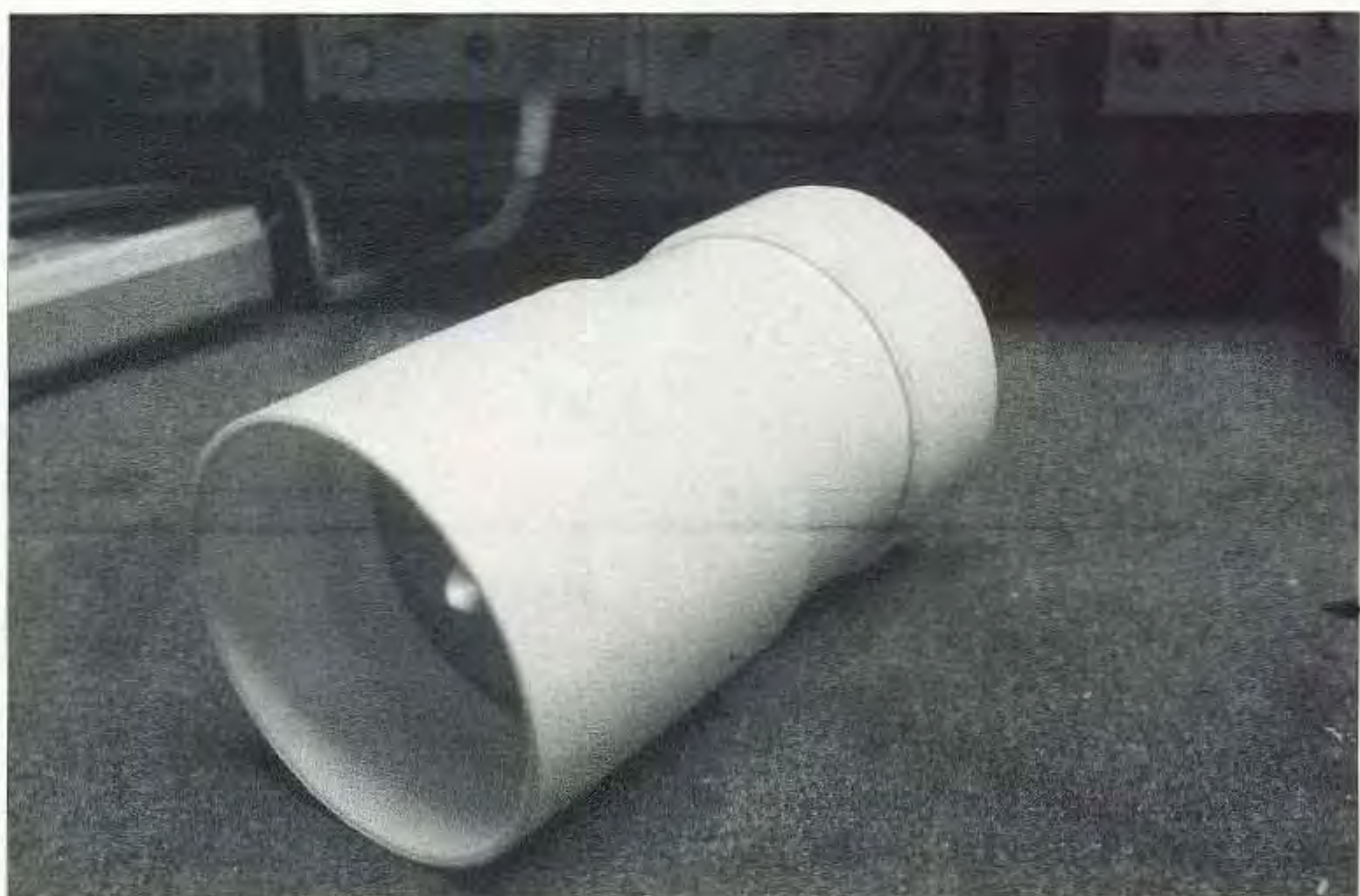
Photo B. Optical reflector in housing with high-output LED in center of reflector. Electronics in rear of housing pipe containing 555 timer chip running at 35 kHz rate to drive LED transmitter. LED used from Hosfelt Electronics, part #25-339; cost, about $5 each (1-800-524-6464). Other LED diodes suitable.
