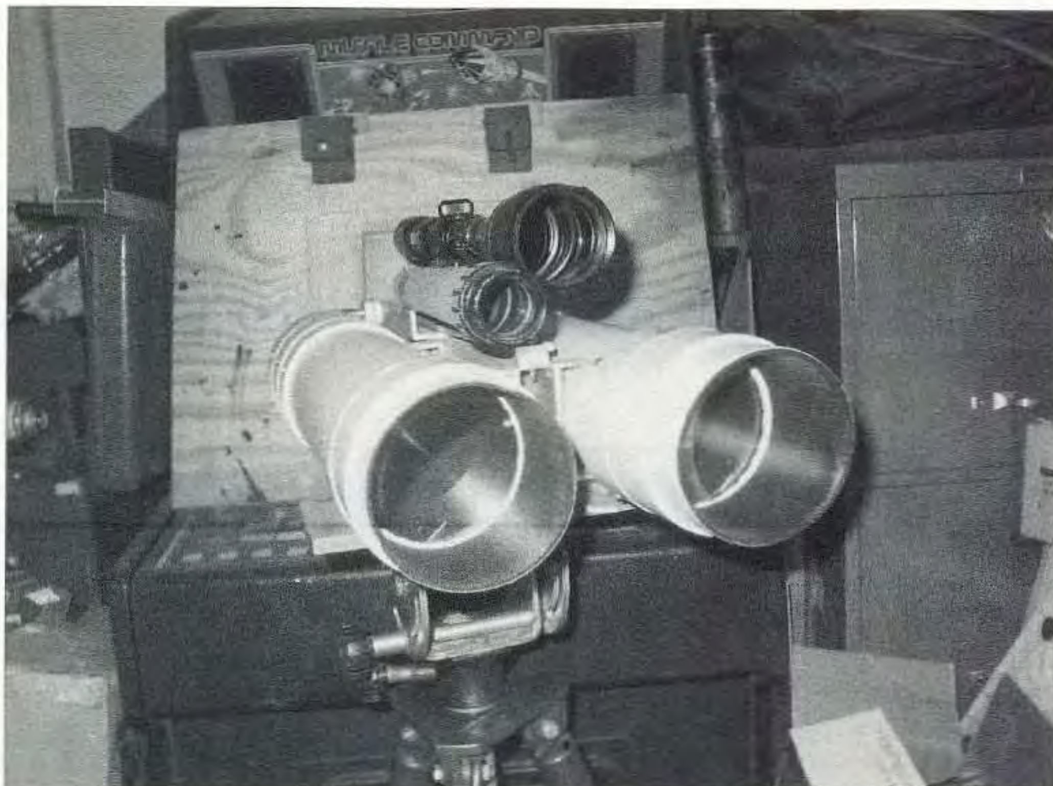
Photo A. Picture of new laser LED transceiver system at WB6IGP. Electronics and 4-inch Fresnel lens inside white 4-inch PVC tubing. PVC coupling sleeves and short sections of pipe and end caps used to create compartments for electronics. Bottom right: photo detector; left: LED transmitter. Top center: spotting scope; just below: laser inside beam expander, laser transmitter.
