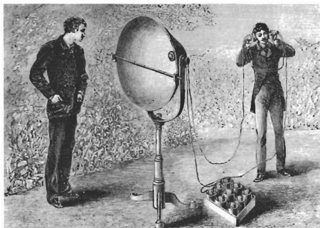
Fig. 2. A photophone receiver of 1880. The detector is the cylindrical object in the reflector.
