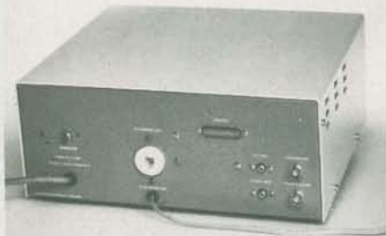
FIG. 17—REAR PANEL of Picture Phone. Circuit-breaker reset is located above line cord at left.
