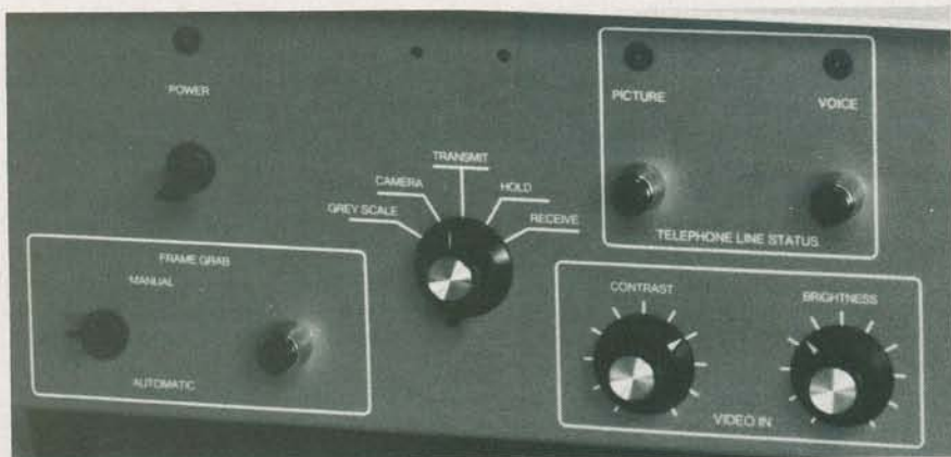
FIG. 21—PICTURE PHONE'S front-panel controls. The FRAME GRAB button is below and to the left of the five-position MODE switch.
