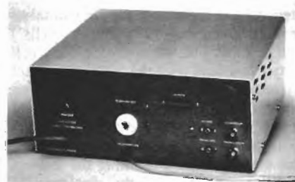
REAR PANEL of Picture Phone. Circuit-breaker reset is located above line cord at left.
