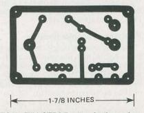
FIG. 4-FULL SIZE foil pattern for the receivercoupler circuit-board.
