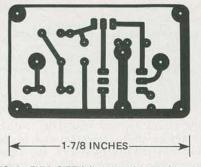
PARTS LIST WIDEBAND ANTENNA PREAMP R1-1 megohm, 1/4 watt C1-1 µF, 25 volts, tantalum Q1-J310 FET (Siliconix or equivalent) NE1-NE99 neon lamp L1-2.2 µH (Mouser 43LS226 or equivalent) T1-Bifilar wound transformer on Amidon FT50-75 core or equivalent (see text) Miscellaneous: PC board, case, coaxial connectors, hardware, etc.
