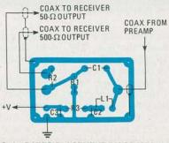
FIG. 6-PARTS-PLACEMENT DIAGRAM for the receiver-coupler board.
