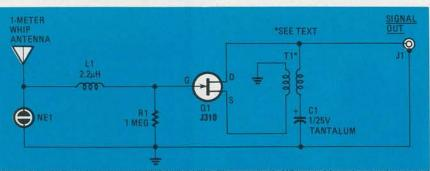
FIG. 1—WIDEBAND PREAMPLIFIER SCHEMATIC. The neon bulb, NE1, provides adequate input static charge protection.
