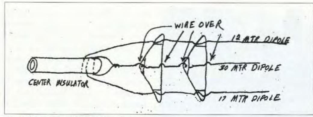
Fig. 3. Wiring detail for clothes hangers.
