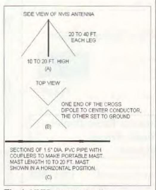
Fig. 1. NVIS antenna details.
