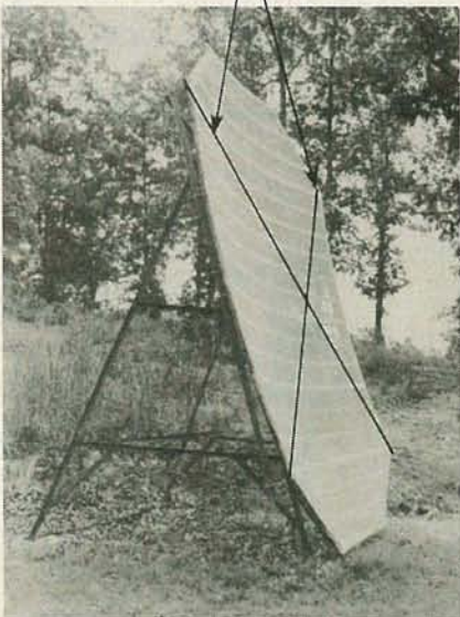
FIG. 32—TWO STRINGS, installed after alignment as shown, make it easy to detect any warps in the reflector surface.
