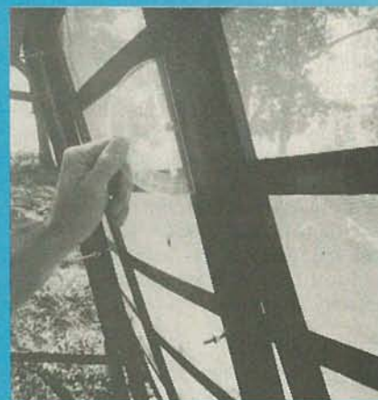
FIG. 27—A SIMPLE INCLINOMETER (a protractor, string, and plumb-bob) used to check the tilt angle of the antenna. With the protractor against a vertical rib, read the angle where the string crosses the scale.
