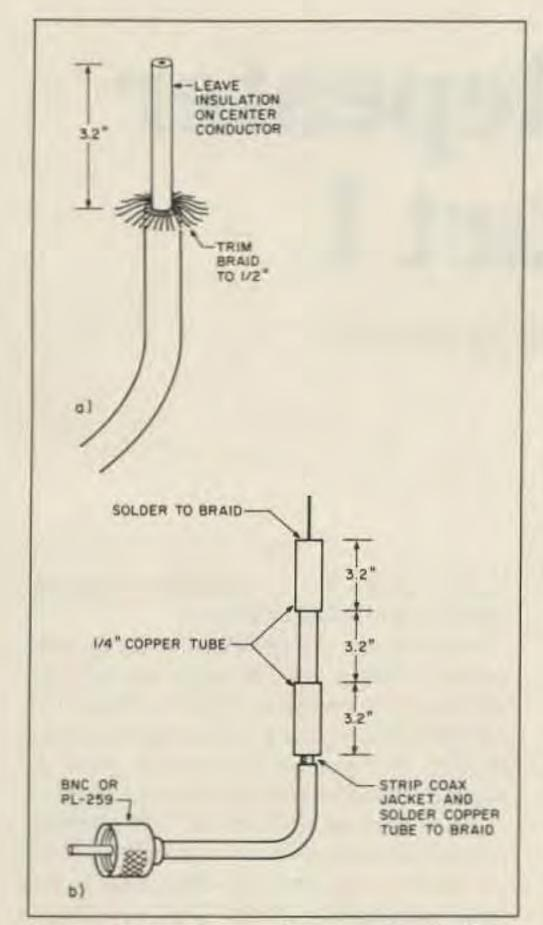
Figure 4. (a) Prepare the coax for the halfwave reference antenna. (b) Attach the sleeve and the RF choke sections of tubing as shown.
