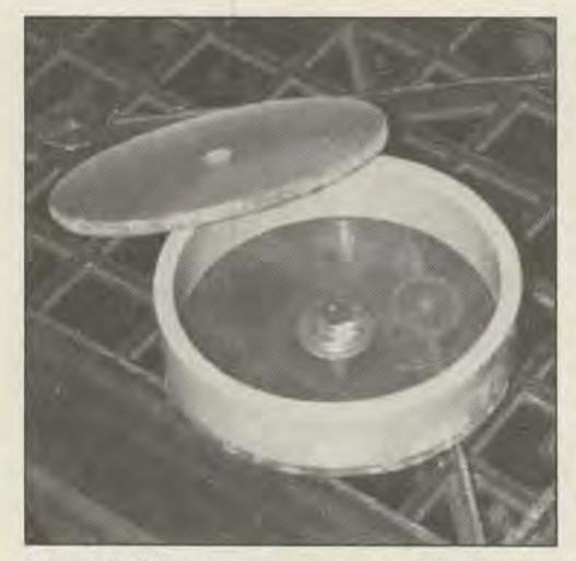
Photo C. The component parts of the loading coil form are made of a slice of PVC pipe with plexiglas end pieces.
