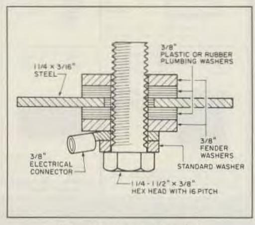
Figure 1. Antenna bracket.
