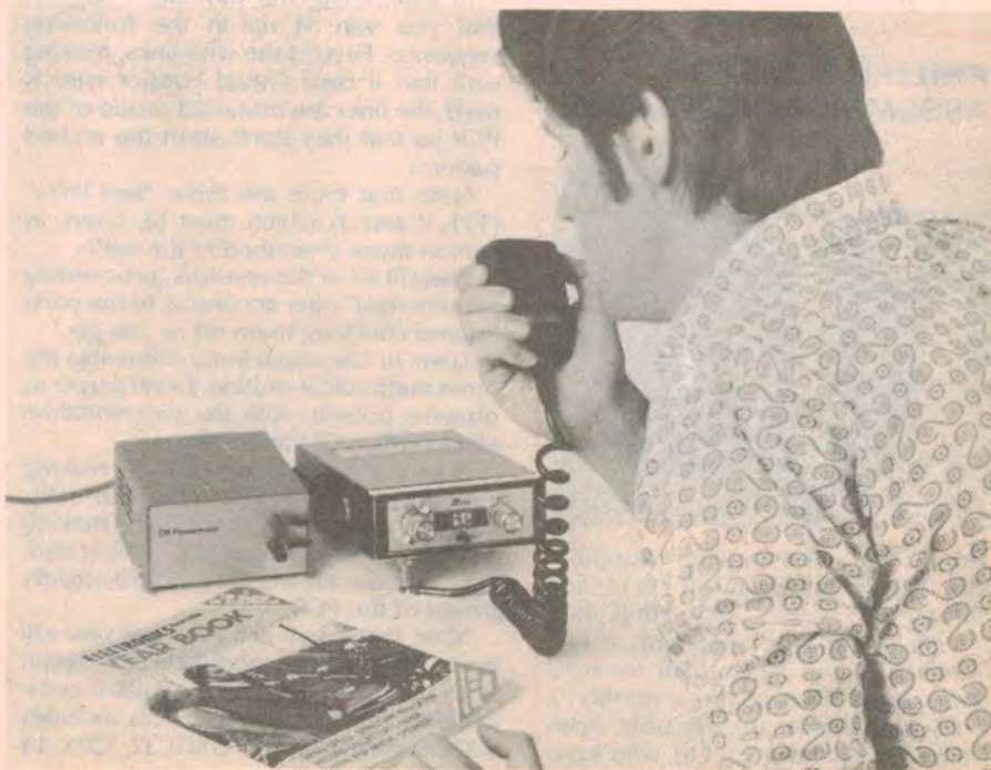
Powermate will run most CB transceivers with a maximum output rating of 5W.
