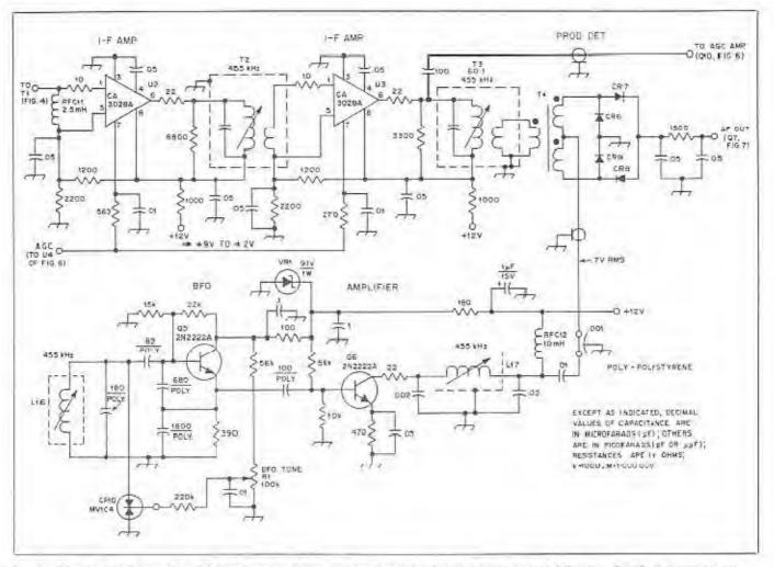
Fig. 5 – Circuit of the i-f amplifier, BF0, and product detector. Capacitors are disk ceramic unless noted differently. Fixed-value resistors are 1/2-W composition. Dashed lines show shield enclosures. The BFO and i-f circuits are installed in separate shield boxes. The R-C active filter and all preamplifier are on a common circuit board, which is not shielded.
