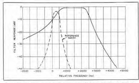
Fig 7—Frequency response of a simple three-pole SSB filter. The circuit is that of Fig 2 with all capacitors changed to 30 pF and terminations of 1500 ohms.
