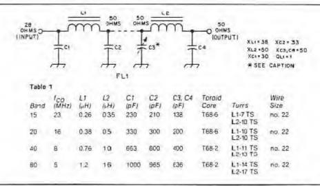
Coil and capacitor information for the half-wave harmonic filters shown in Fig. 1. All capacitors are silver-mica units. Parallel or series combinations can be used as needed to provide the approximate values listed above. An accuracy of ±10 percent is recommended. \*A m ca compression trimmer can be used a C3 to provide final adjustment of the filters.
