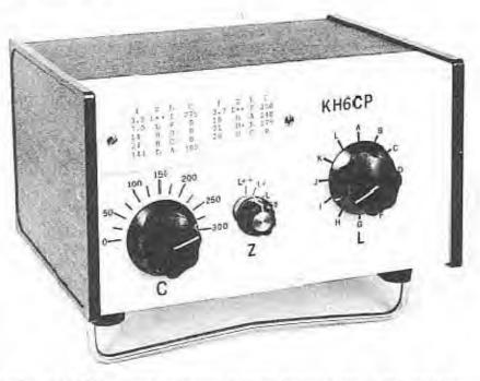
Fig 39 - This ORP Transmatch for balanced feed lines features a balun at the input of the matching network.
