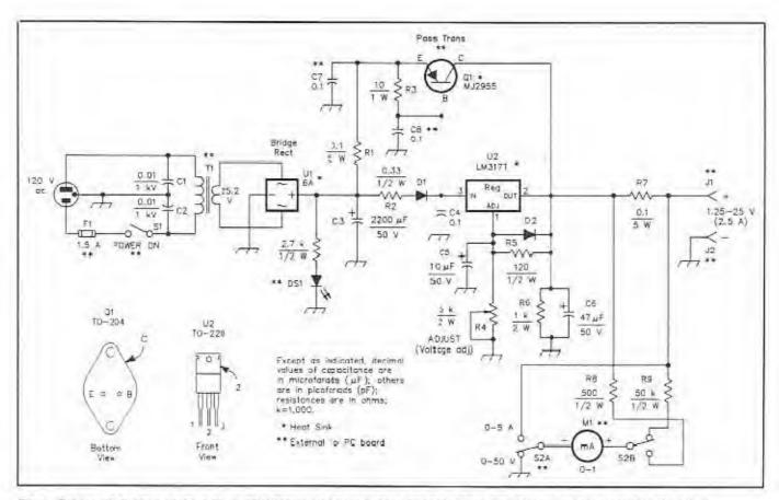
Fig 1—Schematic diagram of the 1.25 to 25-V regulated power supply. Capacitors are disc ceramic except for those with polarity marked, which are electrolytic. See text for data concerning heat sinks for Q1, U2 and U3.
