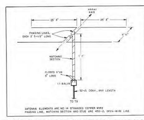
Fig 7—Proposed alternative method of phasing two EDZs. In this arrangement, the length of each phasing line is half the EDZ spacing. Calculated impedance across points a and b is 15/112  $\Omega$ . The matching section—11° in length—transforms this to a calculated impedance of approximately 55-/32 Ω (balanced) across points x and y. The stub, 4 " long, cancels the capacitive reactance (32 0). A 1:1 balun transformer allows the array to be fed by means of 52-Ω coaxial cable. See text.
