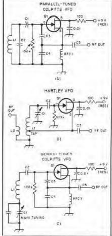
Fig. 4 — Examples of coll-capacitor oscillators (see text).
