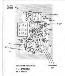
Fig 3—Parts-placement guide for the VFO, not to scale. Parts are placed on the nonfoil side of the board; the shaded area represents an X-ray view of the copper pattern. In the interest of stability, do not use double-sided board material and a ground plane. Component outlines are not necessarily representative of the shapes of the actual parts used.
