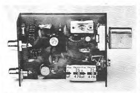
Fig. 7 — Photograph of the assembled kit version (note 7) of the W7ZOI GRP transmitter, as faid out and built by WA&UZO. The panels are made from pieces of double-sided pc board. The dimensions (HWD) are 7/8  $\times$  2-1/4  $\times$  3 inches (22  $\times$  57  $\times$  76 mm).
