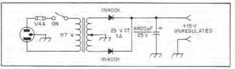
Fig. 10-Schematic diagram of the unregulated power supply.
