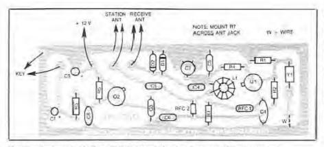
Fig. 7 Component side view of the PC board showing placement of the components.
