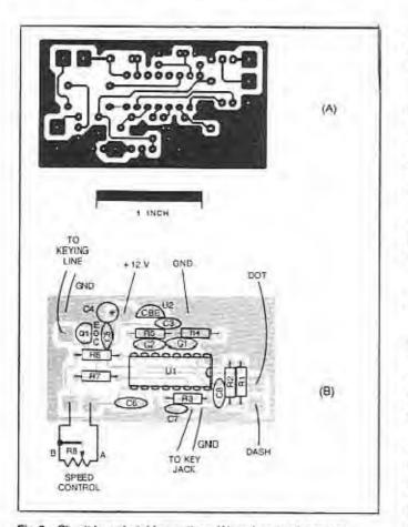
Fig 3—Circuit-board etching pattern (A) and parts-placement guide (B) for the keyer. The pattern is shown full-size from the foil side of the board. Black areas represent unetched copper foil. Parts are placed on the nonfoil side of the board; the shaded area represents an X-ray view of the copper pattern. center. The end insulators are made so that element lengths can be adjusted easily for changing bands.
