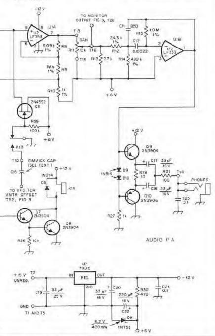
T25-2 core; secondary 28 turns no. 30. T3. T4—15 turns no. 30 trilliar wound on Amidon FT-50-43 core or part of U3 (see text).
