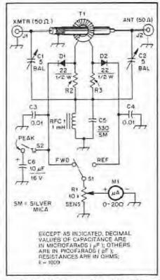
Fig 5-Hybrid diagram of the QRO SWR bridge. A short length of 60 ohm coaxial cable is passed through the center of toroid T1, as indicated. Fixed-value resistors are 1/2-W carbon-composition types. Other components are described below. Radio Shack numbers included.
