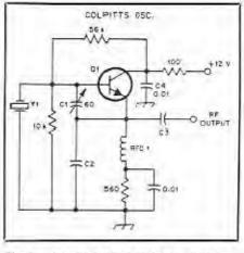
Fig. 2 — A basic Colpitts oscillator using a crystal.
