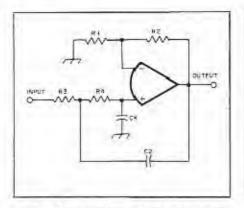
Fig. 9 — A low-pass active litter Finr O greater than one, a low pass filter has a peak in the frequency response similar to that of a band pass filter. For relatively narrow bandwidths, O is approximately  $I_0(B, B2)R1 = 2 - (1/D)$ , For a given value of C (C1 = C2), R3 = R4 = 11/2nt\_0C), where R is in k0, C is in  $\mu$ F, and  $I_0$  is in kHz. The gain at  $I_0$  is 3D = 1.
