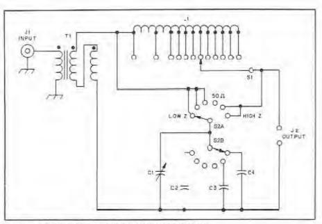
Fig 40 - Schematic diagram of the QRP Balanced Transmatch.
