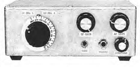
Fig. 1 — The band-imaging receiver covers the CW segments of the 10- and 18-MHz amateur bands with good stability, sensitivity and single-signa selectivity. Larger controls are (I-r) TUNING, IF GAIN and AF GAIN. The two smaller controls, separated by the PHONES jack, are BAND and SIDETONE LEVEL. The TUNING scale is drawn on contact paper applied to an aluminum disc.
