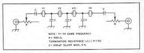
Fig B-Schematic diagram of the crystal filters. Capacitors are all of equal value. Terminating resistors are variable 500-ohm units. Crystals are all of ecual nominal frequency with minor (up to 50-Hz) variation
