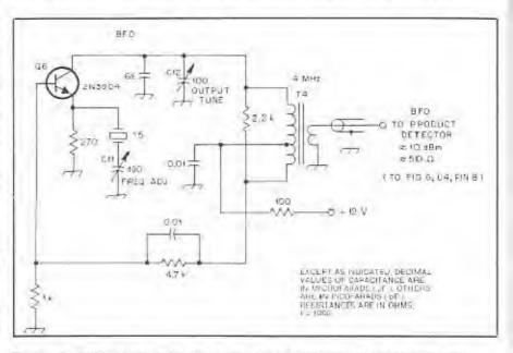
Fig. 5 - Schematic of the band-imaging receiver BFO. Capacitors are disc ceramic unless otherwise noted. Capacitors marked with polarity are electrolytic. All resistors are 1/4-W, 10% units unless otherwise noted
