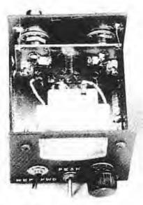
Fig 6-Interior view of the ORO SWR bridge. The PC board is attached to the solder terminals of the BNC jacks. The bottom edge of the PC board is soldered to the chassis at the center. Short wires (upper right and left of PC board) ground the board to the rear panel of the box. C1 and C2 are on the stched-foil side of the board to permit easy access during bridge adjustment (nulling).
