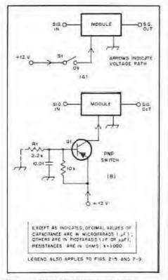
Fig. 1 — Comparison between a simple mechanical switch and an equivalent solidstate type.
