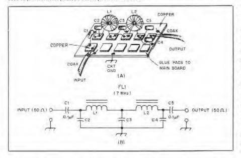
components are installed. A small amount of copper is removed around each peboard hole to prevent short-circuiting the component leads to the ground plane.
