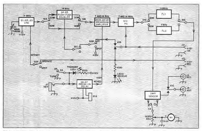
Fig. 1 — Block diagram of the two-band, solid-state transmitter. The arrow heads indicate the direction of signal or do voltage flow. Coaxial cable (miniature) should be used between the various modules when completing signal paths. S1 is a five-pole, two-position, wa'er switch with phenolic insulation. S2 is a dpdt miniature toggle switch. S3 and S4 are spst miniature toggle switches.
