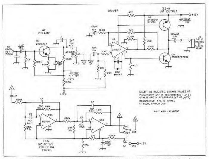
Fig. 7 - Diagram of the audio amplifier and R-C active filter. Capacitors are disk ceramic unless otherwise noted. Polarized capacitors are electrolytic or tantalum. Fixed-value resistors are 1/2-W composition. This circuit is not contained in a shield box. Heat sinks are used with Q8 and Q9.
