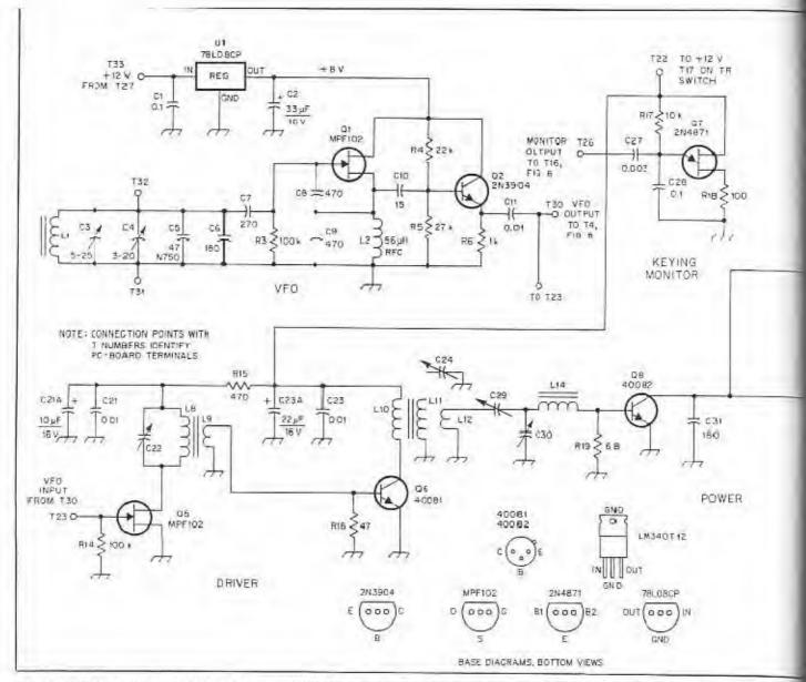
Fig. 9 - Schamatic diagram of the VFO and modified MAVTI-40 transmitter. Components are numbered to agree with those of the original MAVTI-40 VFO and transmitter. Therefore, designators O3 and O4 are missing. Note: Equivalent parts may be substituted. Unless otherwise specified, enameled wire is used for inductor windings.
