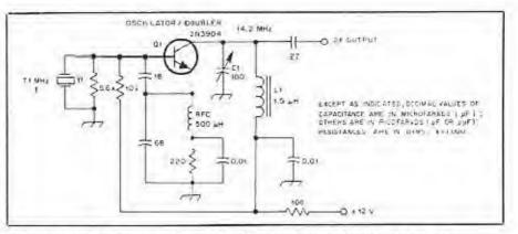
Fig. 2 — A crystal occillator may be used as a frequency multiplier, as shown here. The collector circuit is tuned to the desired harmonic of the crystal.
