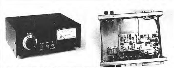
= a. 47 - The completed 6-W VXO controlled transmitter is housed in a small aluminum enclosure. RG-174 is used for all interconnections carrying RF. This version uses the older MRF472 output transistors, which are mounted flat on the boarc.
