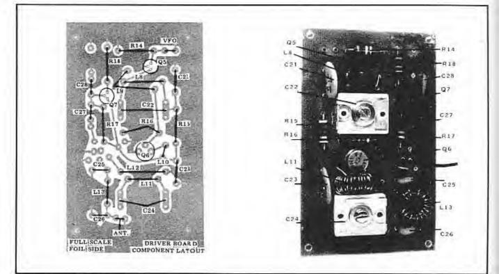
Fig. 6 - Full-size template and parts placement for the driver board.
