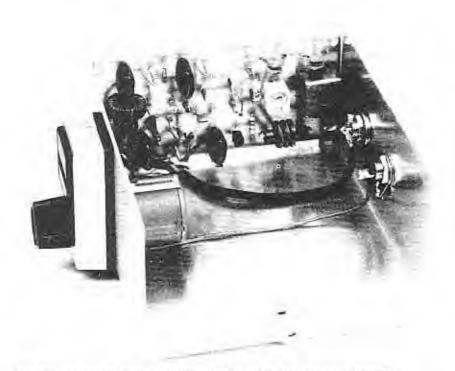
Fig 6-Photographic view of the 40-m VFO in its cabinel with cover removed.
