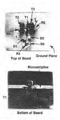
Fig 5—Close-up views of the completed directional coupler. Ti's primary is a straight piece of insulated wire spanning the cut in the microstripline. Ti's secondary winding is routed through the hole cut for T1. The top view shows the components comprising the directional coupler and detector. To achieve minimum lead lengths, R1-R4 are mounted vertically on the ground plane. Capacitors C1 and C2 are not shown, although they should be mounted directly across R3 and R4, respectively.
