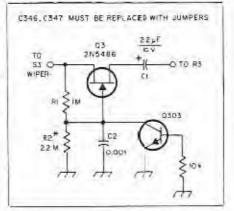
Fig 6—Schematic diagram of the audio thump suppressor. Q303 is part of the transceiver—see text.
