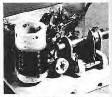
The Vackar oscillator circuit is constructed on a heavy extrusion. Large bus wire interconnacts funed circuit components. Lt is wound on a ceramic form and coated with epoxy resin. C1 is a heavy-duty two-bearing capacitor reduced to one rotor and one stator plate.
