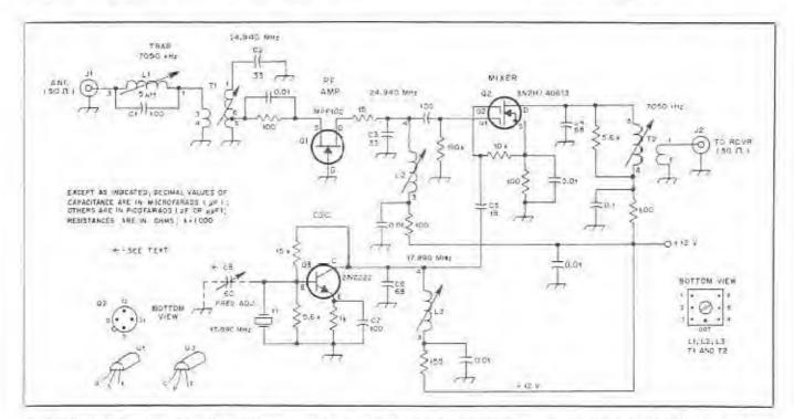
Fig. 2 — Schematic diagram of the 24-MHz receiving converter. Fixed-value capacitors are disc-ceramic, unless otherwise noted. Resistors are 'a- or 32-W carbon-composition.
