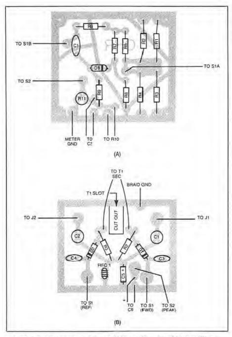
Fig 4-Scale parts-placement guide for the QRP meter (A) and the QRO meter (B), as viewed from the component side of the boards.
