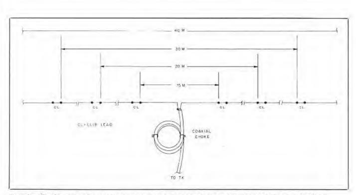
Fig 6—Larry Barry's multiband dipole makes crafty use of clip leads and thumbtacks to stuff half-wave dipoles for 15, 20, 30 and 40 meters into cramped apartment space. Changing bands entails only the connection or disconnection of clip leads. This drawing shows a straight dipole; Larry's antenna is bent into a square but works just fine. See text.
