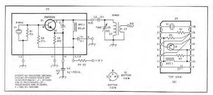
Fig 3—Example (A) of a crystal oscillator that can be built on an IC header. The heavy black line indicates the MCM boundary. All other parts are external to the MCM. L1 is a 5.5-µH inductor (33 turns of no. 28 enameled wire on an Amidon T50-2 core). L2 consists of 6 turns of no. 28 wire. The MCM layout is given at B.
