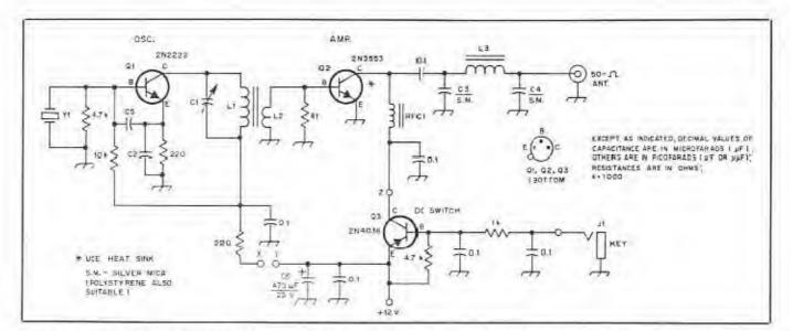
Fig. 5 — Circuit of the W7ZOI "Universal ORP Transmitter." It can provide up to 1.5 watts of rf output when using a 12- to 14-volt dc supply. Fixedvalue capacitors are disc ceramic unless otherwise indicated. Resitors are 1/4- or 1/2-watt composition, 10% tolerance. Values not given are listed in Table 1. C6 is electrolytic or lantalum. C1 is a mica trimmer. O2 is a Motorola transistor, but other brands and numbers with equivalent characteristics can be used.
