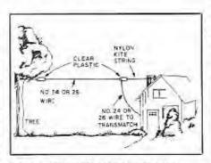
Fig. 2 — Light-gauge enamel-covered wire works nicely as a hard-to-see antenna. Although a bird may knock it down from time to time, recercting it beats having no antenna at all!
