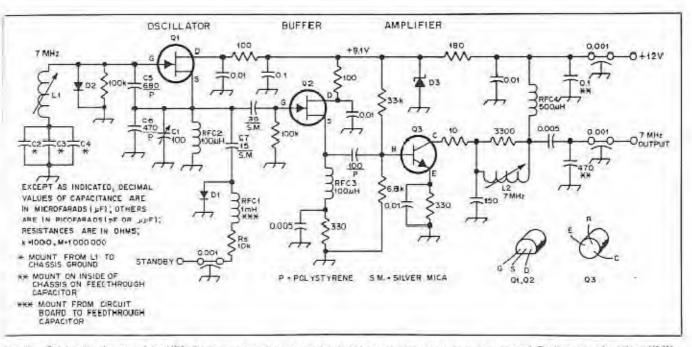
Fig. 2 — Schematic diagram of the VFO. Fixed-value capacitors are disk or chip ceramic unless otherwise indicated. Resistors can be 1/4- or 1/2-W composition. (See June, 1976, ham radio for the author's detailed explanation of this VFO circuit.)
