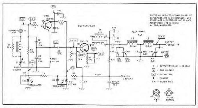
Fig. 7 — Schematic diagram of a universal VXO. Fixed-value capacitors except those in Table 1 are disc ceramic. The polarzed capacitor is tantalum or electrolytic. Resistors other than R3 are ¼- or ½ W carbon composition. R3 is a ½ W unit.
