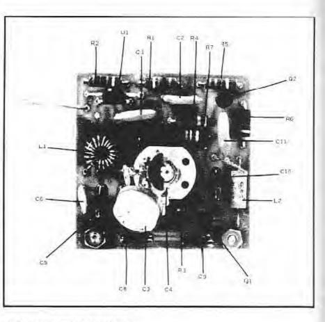
Fig. 5 - Parts placement for the VFO board.
