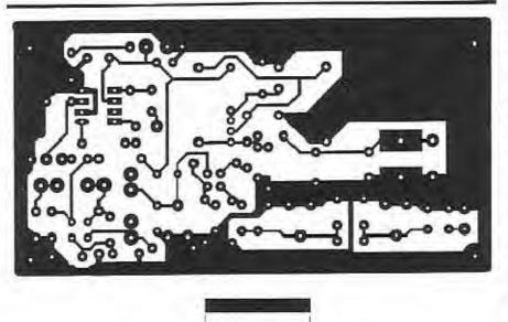
Fig 2-Circuit-board etching pattern for the receiver, shown full-size from the etched side of the boald. Black areas represent unetched copper foil.
