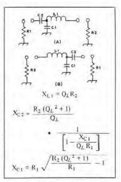
Fig. 3 – Basic circuit for use with Tables 1, 2 and 3. Circuit A, for Tables 1 and 2, shows the network for input matching. B is used n matching the amplifier to 50-ohm output. The formulas are for operating conditions other than those assumed in the tables.
