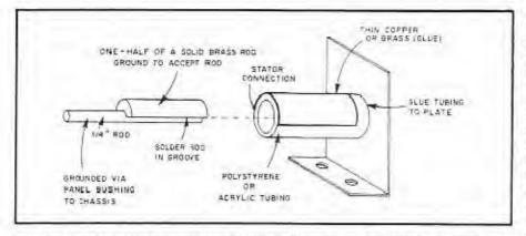
Fig. 5—A cylindrical format provides still another tuning device that can be made at home. The rotor unit is semicircular brass or copper to which a ¼-inch-diameter tuning (od has been soldered. The stator section is a piece of plastic tubing to which thin copper or brass sheeting has been glued (see text).
