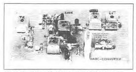
Fig. 1 — The assembled converter. Shleided Amidon Associates L43 and L57 transformer assemblies are used for the tuned circuits.
