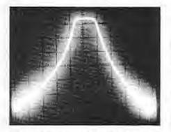
Fig E—Spectral photo showing the response of filter no. 3. Horizontal divisions are each 200 Hz; vertical divisions are each 10 cB. Sampling bandwid/h is 100 Hz. The center frequency is 4.000 MHz.
