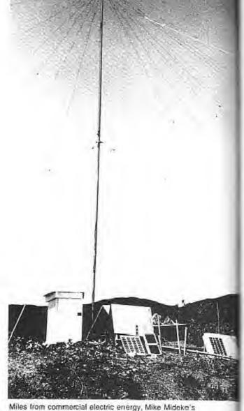
Miles from commercial electric energy, Mike Mideke's experimental 1750-meter beacon has chugged along on solar power since 1984. The antenna is an 18-foot vertical. (photos by WB6EER)
