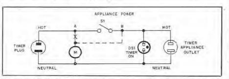
Fig 1—Dennis Cripp's modified timer turns itself and its associated battery charger off at the end of the charging period. Modification of the timer consists of moving the hot motor lead from point A to point B, and installation of a 120-V neon lamp, DS1, between hot and neutral on the timer's appliance outlet.
