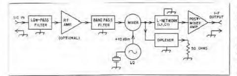
Fig. 1 - Block diagram of the CER-verters.
