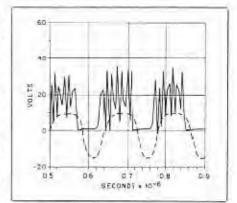
Fig. 3 - When the circuit of Fig. 1 was analyzec on a computer, the waveforms shown were predicted. The solid line indicates how the computer expected the waveform at the collector to look. Expected output wavelorm is shown by the dotted line.
