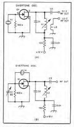
Fig. 3 - Two common types of crystal overtone oscillator.
