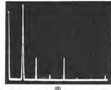
Fig. 6 — Spectral display of the ORP transmitter, without the filter (A) and with the filter (B). Horizontal divisions are each 10 MHz; vertical divisions are each 10 dB. Power output is approximately 0.25 W on 20 meters. At A, all spurious cutput is at least 34 dB down from peak fundamental output; at B, at least 52 dB down.
