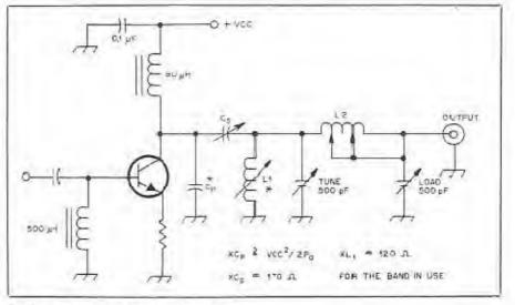
Fig. 2 - Details of the parallel-resonant circuit
