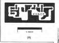
Fig 8—Circuit-board etching pattern (A) and parts-placement guide (B) for the audio thump suppressor and meter switch circuit. The pattern is shown full-size from the foil side of the board. Black areas represent unetched copper foil. Parts are placed on the nonfoil side of the board; the shaded area represents an X-ray view of the copper pattern.
