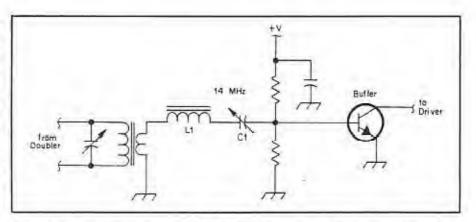
Fig 3—Bob Kuehn added this 14-MHz series-resonant circuit (L1C1) to clean up the output of a push-push doubler in his homemade QRP transmitter. L1 consists of 44 turns of no. 24 enameled wire on a T-68-2 powdered-iron toroidal core. C1 is a small air-dielectric capacitor capable of being set to about 11.5 pF.
