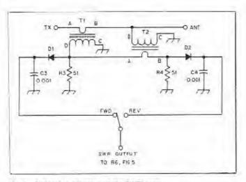
Fig 4—Schematic diagram of the SWR meter. D1, D2—Shotky diode HP 2800-2635 (1N34A can be substituted).
