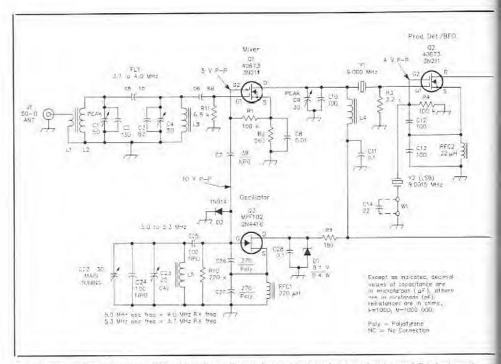
Fig 1—Schematic diagram of the simple SSR receiver. Fixed-value capacitors are disc ceramic unless otherwise roted. Polarized capacitors are tantalum or electrolytic. Fixed-value resistors are ¼-W carbon composition.
