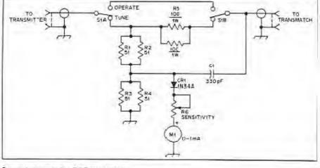
Protective circuit for QRP transmitters.
