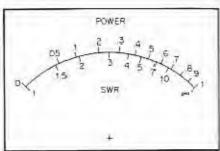
Fig 2—Example of a finished meter face. This scale is that of the meter used in "A Simple and Accurate ORP Directional Wattmeter".
