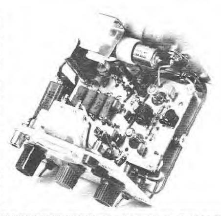
Fig 3—Interior view of the assembled Omni Box. The battery holders are affixed to the rear wall of the cabinet. The SWR bridge is at the far right of the PC heard. The field-strength meter and dummy load are near the front panel at the left side of the cabinet. <sup>V1</sup> and the 100-kHz oscillator are located below the batteries.
