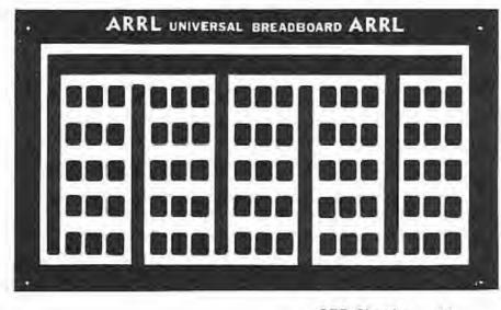
Black represents copper; the pattern is shown at actual size. The board is single sided (copper on one side only), shown from the foil side, and is a Universal breadboard pattern suggested by DeMaw (see Fig 5).
