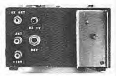
Rear view of the W1FB version of the transmitter. The heat sink is at the far right. The phono jacks and key jack are grouped at the left.
