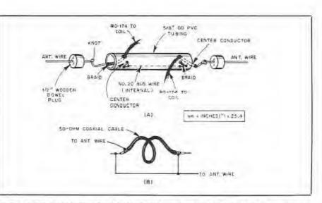
Fig. 9 - At A is a breakaway view of a coaxial trap. The Illustration at B shows the electrical connections for a coaxial trap.
