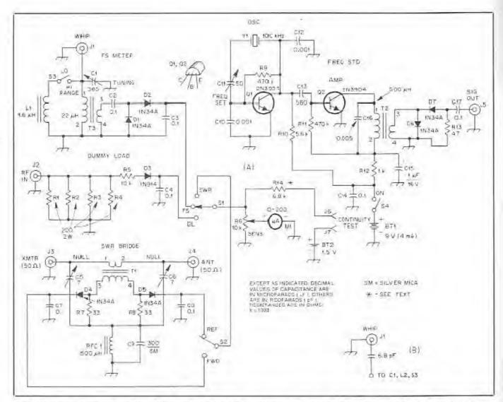
Fig 1—Schematic diagram of the Omni Box circuits. Fixed-value capacitors are miniature chip or disc ceramic types, except for C15, which is electrolytic. Fixed-value resistors are ¼-W carbon composition except for R1-R4, incl, which are 2-W units. Numbered parts that do not appear in the parts list are identified for circuit board layout convenience.
