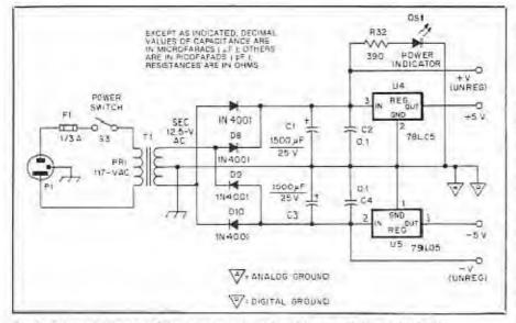
Fig 4—Schematic diagram of the power supply designed for use with the SuperSCAF. D7-D10, Incl—1N4001. T1—117-V pri; 12.5-V sec, 1A (FIS 273-1505 or
