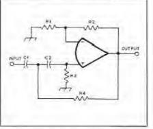
Fig. 11 — A high-pass liller. For farly narrow bandwidth (high Q), the Q of a high-pass liller is approximately  $f_0/B$ , R2/R1 = 2 – (1/Q). For a given value or C (C1 = C2), R3 = R4 = 1/(2nl\_0C), where all quantities are expressed in the same units used in the previous examples. The gain at  $f_c$  is 3Q – 1
