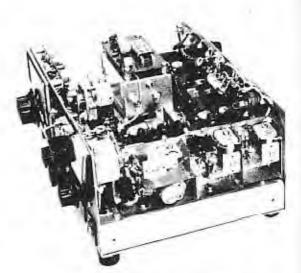
Side view of the K1ZJH 50-MHz transceiver, with cover removed, showing the transmitter of emplifier stages, not completely seen in the top view, Part 1.
