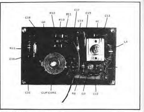
Fig. 2 - Parts placement for the receiver board.
