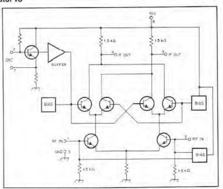
Fig A-The equivalent circuit of the NE602 coubly balanced mixer/oscillator IC.
