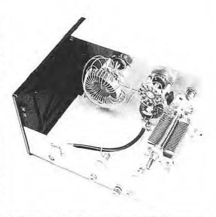
Fig. 41 — Interior layout of the ORP Transmatch. The variable capacitor is mounted on a Plexiglas block.
