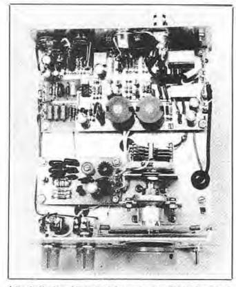
A top, inside view of the author's transceiver. The VFC PC board is at the front left, behind the GAIN and NULL potentiometers. The receiver board is at the rear of the unit. At the front right-hand side of the board is the doubly balanced mixer module. Almost directly behind it, near the rear panel, is the TR relay. The two cylindrical objects at the front center of the board are L1 and L2.
