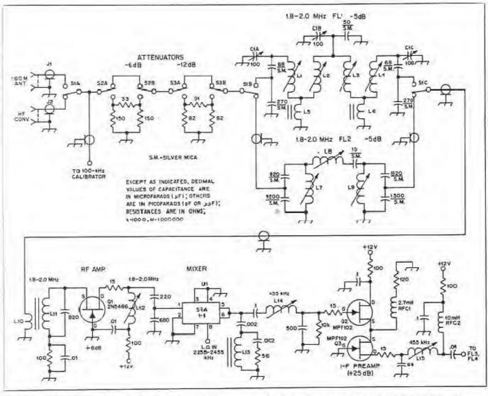
Fig. 1 - Schematic diagram of the receiver front end. Fixed-value apacitors are disk ceramic unless otherwise noted. Resistors C1 - Three-section variable, 100 pF per
