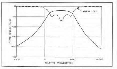
Fig 3—Frequency response of the filter of Fig 2. The dots show the nput return loss, indicating the quality of the mpedance match.
