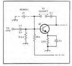
Fig. 4 — Method for attaching a VFO to the circuits of Fig. 1 and Fig. 3. O1 is thus changed from an oscillator to an amplifier.
