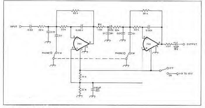
Fig. 16 - A combination phone and cw audio filter.
