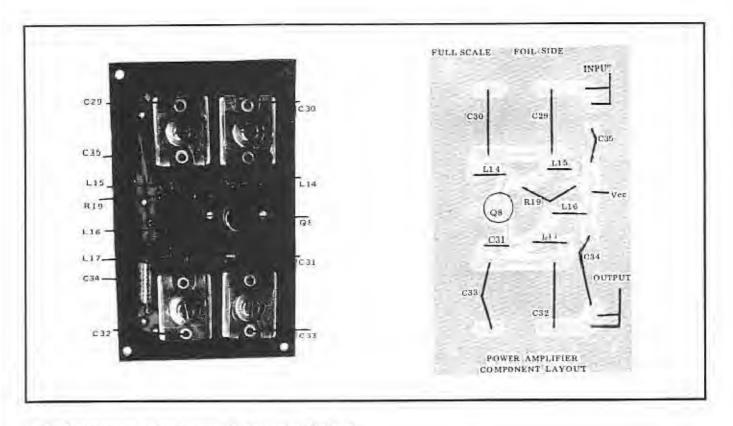
Fig. 7 - Full-size template and parts placement for the power-amplifier board.
