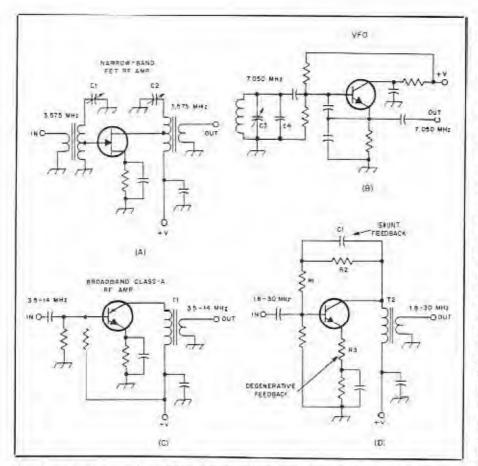
Fig. 1 — The diagrams at A and B illustrate narrow-band amplifiers. The VFO circuit is still a form of amplifier, since its output power (in part) is fed back to the input for the purpose of causing oscillation. A simple Class-A broadband amplifier without feedback is seen at C. A fedback Class-A broadband amplifier is shown at D. It uses a combination of shunt and degenerative feedback (see text).
