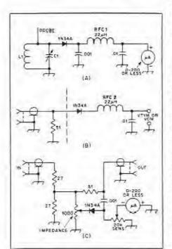
Fig. 2 — Simple tes: equipment used in optimizing the solid-state amplifier includes a wavemeter, A, a power-output indicator, B, and a variable impedance bridge, C. Values of L1 and C1 depend on the band being checked. Parts designations are for text reference.
