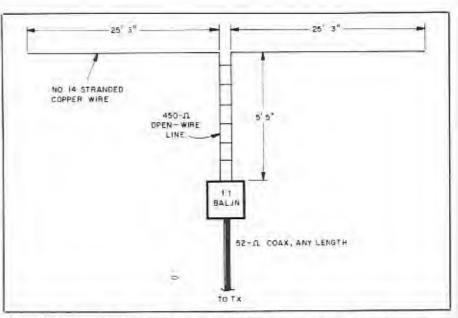
Fig 3—The extended double Zepp at K7KGP, but for 24.950 MHz. The 450- $\Omega$  matching section transforms the EDZ's calculated input impedance (142-/555  $\Omega$ ) to 55  $\Omega$  (measured) for connection to 52- $\Omega$  coaxial cable by means of a 1:1 balun. The electrical length of the matching section is 52°; the linear dimension shown in the drawing assumes 450- $\Omega$  line with a velocity factor of 0.95.
