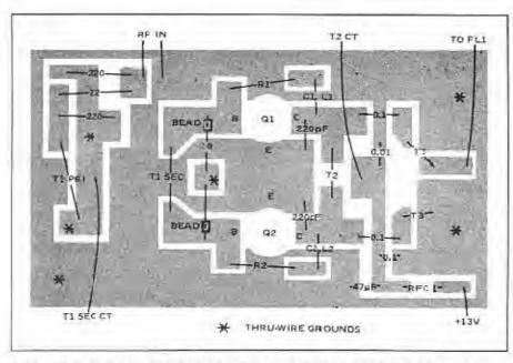
Fig. 2 — Parts placement guide for the amplifier board. Parts are mounted on the etched side of the double-sided pc board; the shaded area in this view represents the copper pattern. The other side of the board is unetched. Decimal-value numbers alone represent capacitance in microfarads. Whole-number values without units represent resistance in ohms. Note that ferrile beads are slipped over one end of each of the two 10-ohm resistors.
