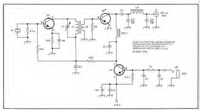
Fig 1—A schematic diagram of the QRP transmitter for 30-meter operation, Fixed-value capacitors are disc ceramic, Inductor cores are available from Amidon Associates or Palomar Engineers.<sup>1,2</sup> The enclosure is from Radio Shack<sup>s</sup> (RS-270-251), and the circuit board is from Circuit Board Specialis's.3 An etching pattern for this circuit appears on p 11.
