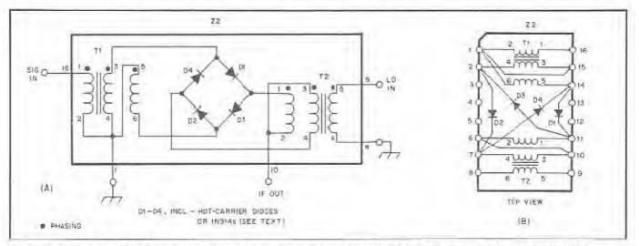
Fig 2—Circuit for a doubly balanced mixer, balanced modulator or product detector. Matched diodes are necessary for best DBM balance. Hct-carrier diodes are recommended for this circuit, but matched 1N914s are suitable. T1 and T2 in my MCM consist of four trifilar turns of no. 30 enameled wire through an Amdon balun core no. BN-43-2402. An FT-23-43 ferrite toroid core may be substituted (smaller) by winding 7 trifilar turns of no. 30 enameled wire on each core.
