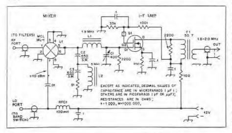
rf inputs. The difference frequency is used to drive the WICER receiver. However, a termination must also be provided for the sum frequency.
