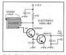
Fig. 5 — Practical circuit for an electronic hand key. The etched/oil grid at the left is the keying contact. Transmitter or code-practice oscillator keying occurs when the operator places his or her finger on the copper grid. The resistor is in ohms, and the capacitors are n microfarads.
