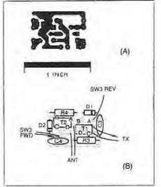
Fig 7—Circuit-board etching pattern (A) and parts-placement guide (B) for the SWR meter. The pattern is shown full-size from the foil side of the board. Black areas represent unetched copper foil. Parts are placed on the nonfoil side of the board; the shaded area represents an X-ray view of the copper pattern.
