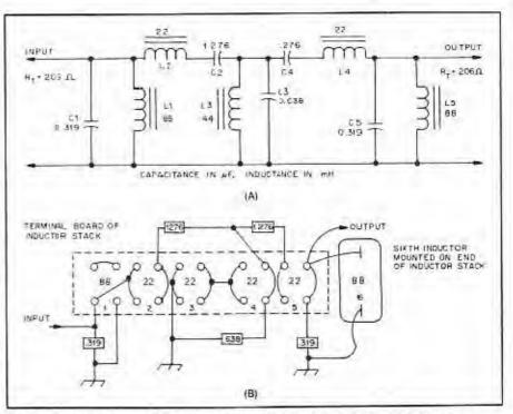
Fig 4—Schematic diagram of the SSB band-pass filter (A). Shown in B is a pictorial wiring diagram of the terminal board on the inductor stack.
