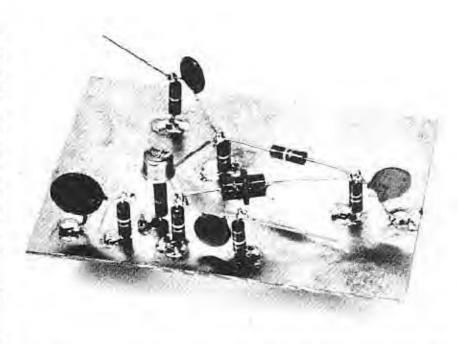
Fig. 1 - Photograph of the simple breadboard depicted in Fig. 2A. High-chmage resistors serve as standoff terminals.
