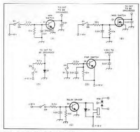
Fig. 4 - Various semiconductor switches (see text).
