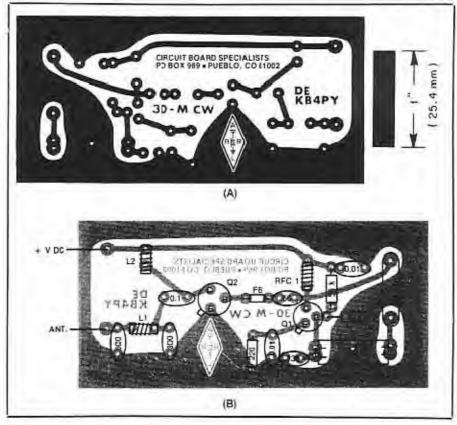
Fig. 3 - A PC-board etching pattern is given at A. Black represents unetched copper, viewed from the foll side of the board. The pattern is shown actual size. B shows a parts placement diagram. Components are placed on the non-foll side of the board; the shaded area represents an X-ray view of the copper pattern.
