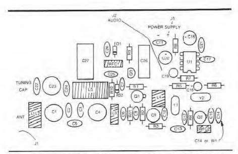
Fig 3-Parts-placement guide for the receiver Parts are placed on the nonfoil side of the board; the shaded area represents an X-ray view of the copper pattern. Component outlines are not necessarily representative of the shapes of the actual parls used.
