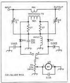
Fig. 12 — Gircuit for the SWR sensor (see text). Fixed-value capacitors are disk caramic. Fixed-value resistors are 1/2-W composition. C11, C12 — 5-pF air variable, pc-board mount. D10, D11 — 1N270 or 1N34A diode. M1 — Small microampere meter. A 50-, 100-
