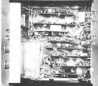
SB generation occurs in the circuit shown in Fig 4. A microphone amplifier (Q16-U6) supplies audio to an MC1496 balanced modulator (U7). Onemicrofarad capacitors (C6-C8) are used at the output of the audio amplifier and at several positions in the balanced modulator. (Originally, 10- or 22-µF units were used, but these caused the system to respond slowly during TR transitions.)
