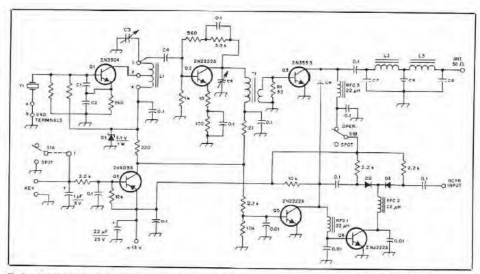
Fig. 9 — A somewhat elegant TR switching method that uses a series diode switch and a signal shunting transistor (Q5, D2 and D3). An explanation is given in the text. This is purely an illustrative RF circuit from Q1 through Q3. Therefore, there is no parts list.
