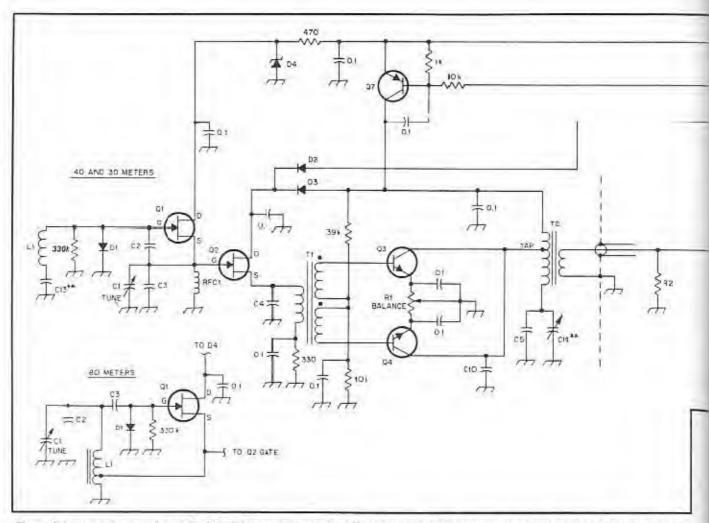
Fig 1-Schematic diagram of the MOuSeFFT low-power transmitter. The 80-meter VFO is shown in the inset drawing. Refer to the parts list and Tables 1 and 2 for parts values not shown on the diagram. All 0.1-#F capacitors are 25-V X7R or Z5U ceramic types. All resistors are 1/4- or 1/2-W, 10% tolerance acceptable.
