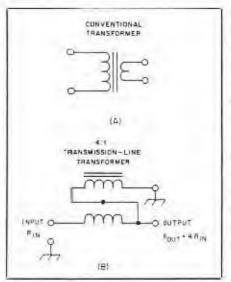
Fig. 3 — Examples of conventiona and transmission-line transformers. See text for additional information.
