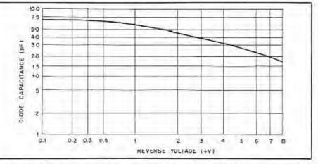
Fig 3—Abbreviated capacitance/reverse voltage curve for an MV2109 tuning diode. Note the flat portion of the curve to the left (see text for precautions about reverse voltages from 0.1 to 1.5).
