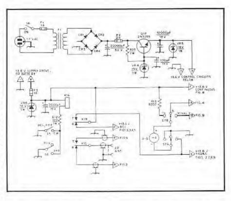
Fig. 10 - Schematic diagram of the power supply and episted circuits for the SQ MHz transcerver, Capacitors are electrolytic, values in µF.
