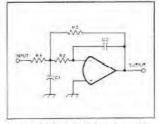
Fig. 10 — Another low-pass filter. Choose C2 then C1 =  $C2(3\Omega)^2$  R1 = R2 = R3 =  $1/(2\pi t_0 \sqrt{C1C2})$ , where R is im k(2 C is in  $\mu$ F and  $t_0$  is in kH2. The gain is equal to  $\Omega$
