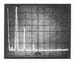
Fig. 11—Spectral display of the transmitter output. Vertical divisions are each 10 dB; horizontal divisions are each 5 MHz. Output power is 4 W at 7 MHz. All spurious emissions are at least 32 dB below peak fundamental output power.
