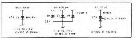
Fig 2—Three types of VVC dodes. A single diode is shown at A. The triple-diode version at B is for tuning three circuits at the same time, such as an RF amplifier, mixer and oscillator. Back-to-back diodes in one package are shown at C.
