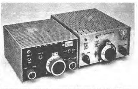
Two versions of the 7- and 14-MHz cw transmitter are shown here. At the left is the WTFB prototype. On the right is a model built by WAØUZO, Both units are small and lightweight.
