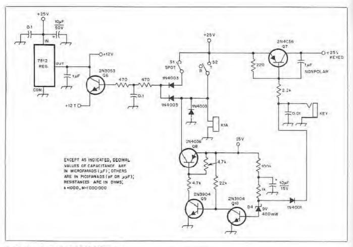
Fig. 2 — Control circuit for the VM0S FET transmitter K1 — 24-V dc spdt relay, Magnecraft D4 W65RPCX-3 or equiv. e
