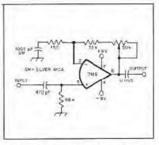
Fig. 13 A 80 kHz band-pass filter. Calculated voltage gain is 200 and the 0 is 10, giving a bandwidth of 5 kHz. Since a standard 741 op amp does not work well above 10 kHz, a high-site w-rate version is used. To design for other frequencies, first choose a value for C1, then  $R2 = (3B/(2nC1)_c^2)$ , where G3 is the gain-bandwidth product of the op amp (1000 kHz for a 741 or 741S). Choose 0 using  $Q = I_0/B$  or Q = GU/(B).
