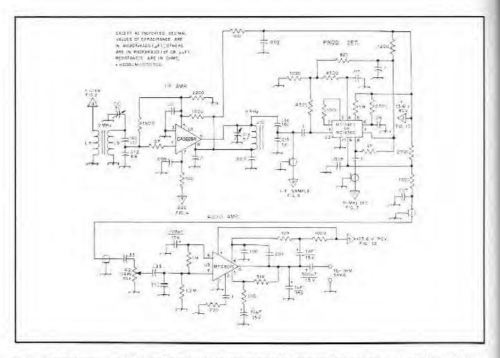
Fig. 3 - Schematic diagram of the 9-MHz i-1 amplifier and product detector, and audio-amplifier modules. Parts not described are numbered for text reference
