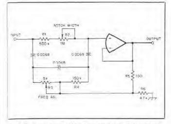
Fig. 3—Schematic diagram of the active notch filter; R3 controls the match frequency. This filter has a gain of 0 dB.
