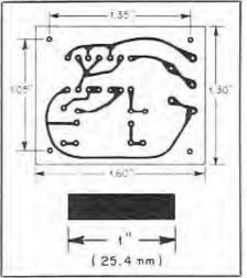
Fig. 4—Full-size circuit-board etching pattern for the frequency marker, shown from the foil side. Black areas represen unetched copper.
