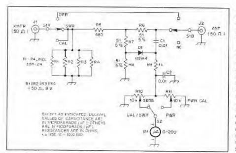
Fig 1—Schematic diagram of the QRP SWR bridge. Resistors are carbon-composition types. Capacitors are disc coramic. Part numbers listed below are Radio Shack designators, except when otherwise noted.
