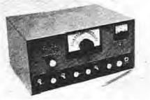
The receiver is built in a homemade aluminum cabinet. A two-tone gray and flatblack paint job has been applied. Black Dymo tape labels are used for identifying the controls in the black area, and gray labels are affixed to the gray portion of the front panel. A cut-flown Jackson Brothers vernier dial mechanism Itwo-speed) is used for frequency readout.
