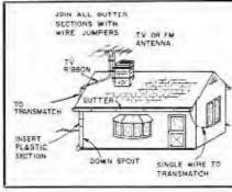
Fig. 3 — Some amateurs have had success when using the rain gutter as a random-length, end-fad radiator. The lower portion should be inaulated from the remainder of the gutter and downspout to prevent rf hazards to animals and people. The TV or im antenna-lead wire also can be used as a random-length antenna, as shown here.
