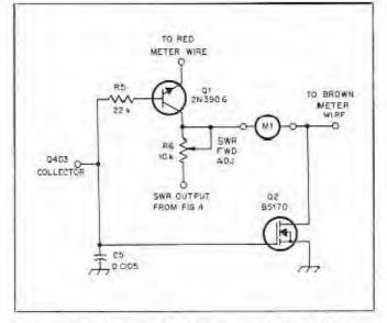
Fig 5—Schematic diagram of the meter switch circuit. Q403 is a Heathkit part designator.
