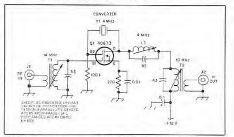
Fig 7—A one-MOSFET converter based on a CQ Ham Radio design. The principal difference between this circuit and that shown in Fig 6 is the drain trap (L1 and the 82-pF capacitor). Solenoidal slug-tuned inductors and transformers were used only because they were hardy; their toroidal equivalents should work as well or better. See text.
