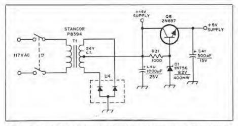
Fig. 3 - Power supply for the heterocyne VFO. Miniature diode assembly U4 is Notorola part no. MDA 950-2 or ecuiv.
