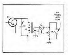
Fig. 2 — Details for measuring transmitter output power with a dummy load (R1), an rf probe and a VOM (see text). homemade rf probe.<sup>3</sup> This will permit us to measure rf voltages in oscillators and transmitters when performing initial checkout or debugging. A frequency counter is very useful to the experimenter, and should be acquired if the expense can be justified.
