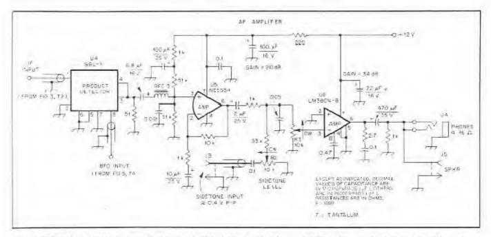
Fig. 5 - Schematic of the product detector and audio amplifiers for the band-imaging receiver, Capacitors are disc ceramic unless otherwise noted. Capacitors marked with polarity are electrolytic. All resistors are 1/4-W, 10% units unless otherwise noted.
