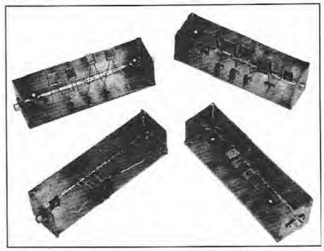
Fig A-Four CW crystal filters were built in this configuration. The PC-board mounting surfaces provide a ground plane. Capacitors are soldered directly to the ground plane and the crystals are connected using the capacitors as standoffs. Phono jacks are used for input and output connectors. The only variables in the construction of the filters are the crystal characteristics and the length of the crystal leads. The SSB filter is not shown.
