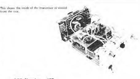
As a matter of interest, the transmitter was operationally checked at  $10^{\circ}F$  increments between  $-40^{\circ}F$  and  $+140^{\circ}F$ . The output was stable and no amplitude change could be observed. Rf power output is typically 5 watts for 8 watts input.
