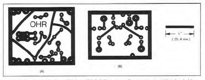
Fig 7-Circuit-board etching patterns for the ORP (A) and ORO (B) SWR/power meters. The patterns are shown full-size from the foil side of the board. Black areas represent unetched copper fcil.
