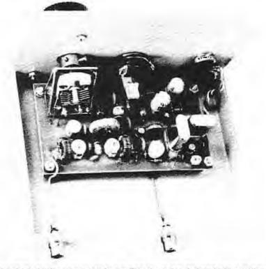
Interior photo showing component layout. This circuit was designed with a minimum number of components, but optional modifications allow 20-meter coverage.
