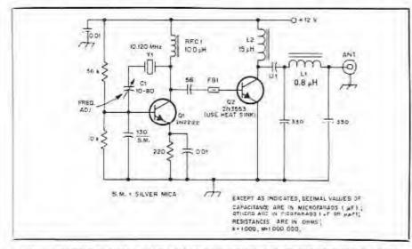
Fig. 1 — Schematic diagram of a simple 30-m transmitter built by KB4PY. Resistors are ¼-W, carbon-composition types. Capacitors are disc ceramic, except C1.
