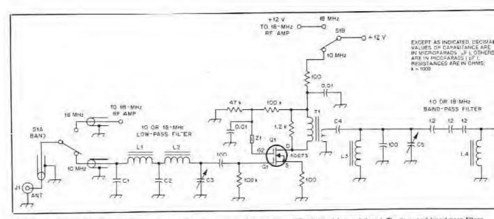
Fig. 2 — Schematic of the RF amplifiers for the band-imaging receiver. A separate amplifier is used for each band. The low- and band-pass filters may be aligned with the aid of a crystal-controlled marker generator; see lext. Capacitors are disc ceramic unless otherwise noted. Capacitors marked with polarity are electrolytic. All resistors are ¼-W, 10% units unless otherwise noted.
