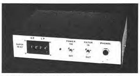
SuperSCAF is a stand-alone unit that contains a switched-capacitor filter, an audio power amplifier and an ac-operated power supply.
