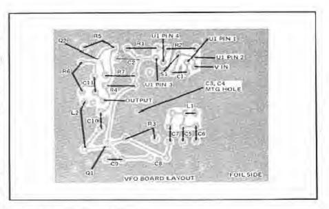
Fig. 4. Full size template for the VFO board.
