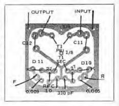
Fig. 13 — Parts placement guide for the SWR sensor, K = the cathode end of a diode. Fractional markings such as "1/8" signify mounting holes to be drilled with that size bit. cover is press-fitted over the box walls. In the author's unit the SWR-sensor module is bolted to the VFO top cover.
