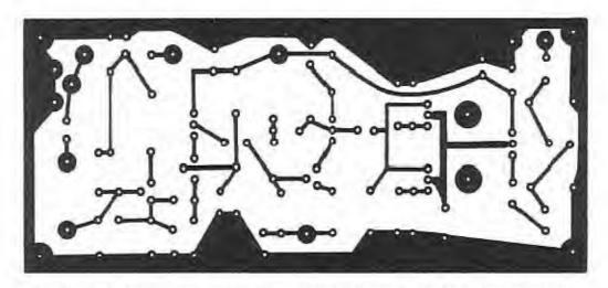
Etching pattern for VXO-controlled CW transmitter. Shown full size from the foll side of the board. Black areas represent unetched copper.
