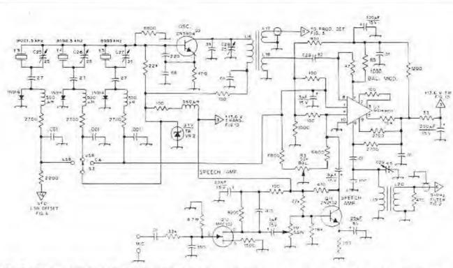
Fig. 7 – Schematic diagram for the sideband generator in the 53-MHz transceiver, Parts not described are numbered for text reference, C25-C28, incl. – Ceramic trimmer, 5 – 25 pF C29 – Ceramic trimmer, 7 – 45 pF L16 – 32 turbs No. 26 Telfon wire on 1/2 inch toroid core (Amidan T-50-2, red)
