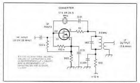
Fig 6—This one-transistor converter stage (RF amplifier not shown) appeared in March 1974 QST. Q1 acts as a Pierce oscillator and mixer. The 10-Q drain resistor may have been included to suppress VHF parasitic oscillations in Q1.
