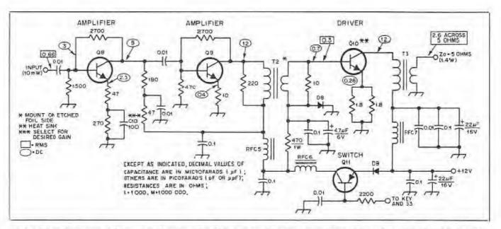
Fig. 7 - Schematic diagram of the prosidend linear emplifier. Opparitors are clak ceramic except those with polarity marked, which are electrolytic or tantalum. Resistors are 1/2-W composition unless otherwise noted. C10 - See text.
