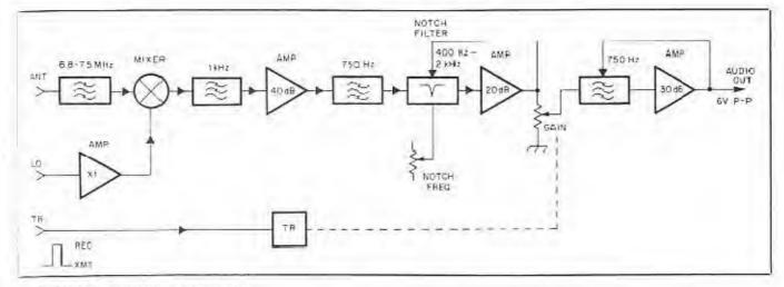
Fig. 5-Block diagram of the new D-C receiver.
