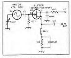
F.g. 6 — Illustration of how a buffer stage can be used after an oscillator to minimize frequency changes caused by load variations.
