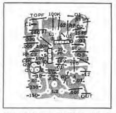
Fig. 3 - Scale layou: of the VFO circuit board showing parts placement from the component side of the board.
