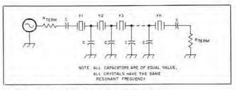
Fig 1-Generalized crystal filler suitable for empirical construction.
