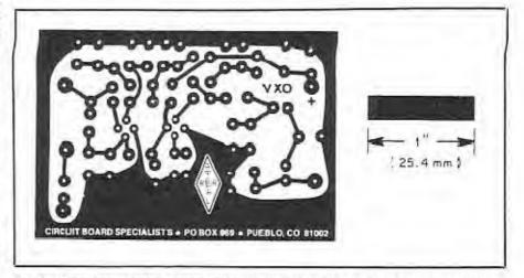
Fig. 9 — Circuit-hoard etching pattern for the Universal VXO. The pattern is shown full-size from the foil side of the board. Black areas represent unetched copper foil.
