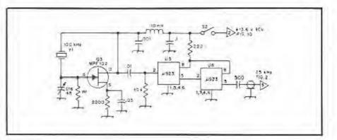
Fig. 5 - Schematic diagram of the 25-kHz crystal calibrator.
