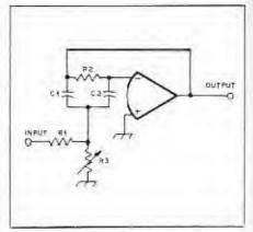
Fig. 6 — A turable band-pass filter. After choosing a value for C (C1 = C2), then R2 = 1/hBC), where R2 is in kII. C is in  $\mu F$ , and B is the bandwidth in kHz. R1 (k0) = R2/2G, where G is the desired numerical voltage gain at resonance.
