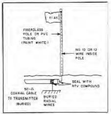
Fig. 4 — One can be patrotic while using a disguised antenna. The flagpole also serves as a vertical antenna in this illustration. Insulation should be used over the lower part of the antenna to prevent shock hazard to people and animals.
