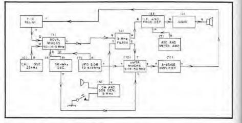
Fig. — Block diagram of the K1ZJH 50-MHz transceiver. Each stem shown is a separate circuit-board assembly. Numbers in paramiteses are the order of their description in the text. Transmitting and receiving functions are given adjacent to the signal-path lines. Items 1 through 6 are described in Part 1.
