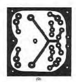
Circuit-board etching patterns for the 7- and 14-MHz cw transmitter (continued). Shown here is the power-amplifier circuit board, which appears in Fig 11, Part 4 of the series. This circuit board is double sided, the component-side foil being used only as a groundplane. That pattern is not shown as it contains only clearance holes for the component leads.
