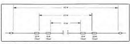
Fig. 1 - Representation of a three-band trap dipole artenna.
