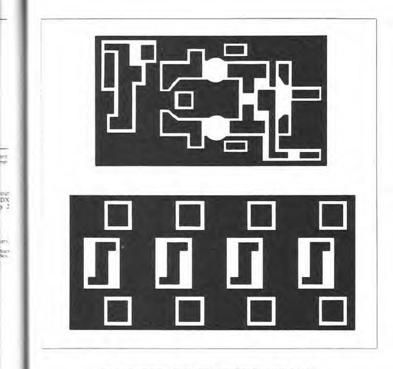
Circuit-board etching patterns. The front sides of the boards are shown here at actual size, with black representing unetched copper. The upper pattern is for the amplifier section (Fig.2): it is copper clad on both sides, with unetched copper on the "back" side that forms a ground plane. The lower pattern is for the filter board (see Fig.3).
