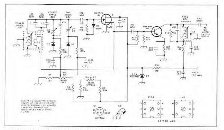
Fig 1—Schematic diagram of the VVC-tuned VFO. Fixed-value capacitors are disc ceramic, 50- or 100-V rating. Fixed value resistors are Va-W carbon composition. NPO notations are for temperature-stable disc capacitors (zero temperature coefficient).
