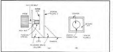
Fig. 4—Mechanical details for a home-made disc tuning capacitor. A tension spring ensures mechanical stability of the rotor portion of the vanable capacitor. Side brackets also help to keep the unit mechanically rigid. The detail at B shows how the stator disc is etched on PC board material.
