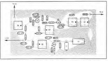
Fig. 3 — Parts-placement guide for the converter, as seen from the component side of the board. The shaded area represents an X-ray view of the copper pattern.
