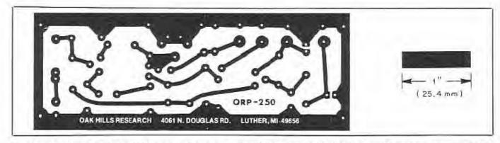
Circuit-board etching pattern for the QRP transmitter. The pattern is shown full size from the foll side of the board. Black areas represent unetched copper foil.
