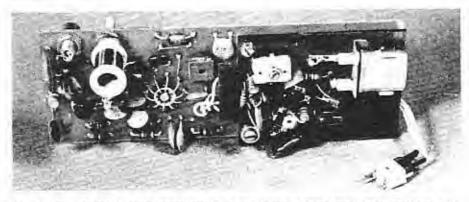
Crystal oscillator and balanced mixer board. The oscillator is a highly modified International AO1 assembly. The small toroid coil on the oscillator board is L2. The balanced mixer (10-lead IC) is on the main board. U2 and Q6 are at far left. As is typical with developmental circuits, the board shows evidence of modifications.
