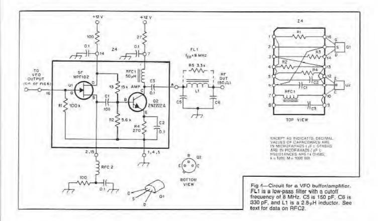
typically. This is par for a source follower. It helps to isolate the VFO from Q2 and the circuits that follow Q2. Amplifier Q2 builds up the VFO energy to a level that is suitable for most circuits with which a VFO is used.
