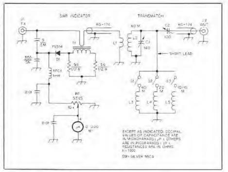
Fig 1—Schematic diagram of the SWR bridge and Transmatch. Fixed-value capacitors are disc ceramic unless noted otherwise. Fixed-value resistors are carbon composition.
