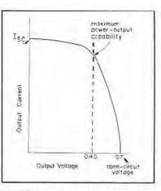
Fig 2—This load curve for a PV solar cell shows that maximum power delivery from a solar cell occurs at approximately 0.45 V output. I<sub>SC</sub> is the short-circut current.
