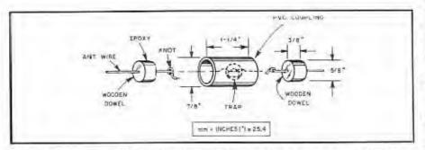
Fig. 6. - Breakaway view of a toroidal mini trap. The knots in the wire prevent stress on the tuned circuit.
