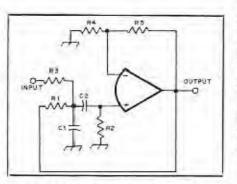
Fig. 3 — An active RC band-pass litter. To design a filter using this circuit, make all the trequency-determining resistors and capacitors equal: R1 = R2 = R3 and C1 = C2, Choose a convenient value for C and then R =  $\sqrt{2}|(2\pi Cf_0)$ , where R is in k0, C is in  $\mu$ F, and  $t_0$  is in kHz. Q =  $f_0/B$ , where B is the 3-dB bandwidth in kHz. R4 and R5 determine the Q: R5/R4 = 3 -( $\sqrt{2}$ /Q). The voltage gain is  $20\sqrt{2} - 1$ .
