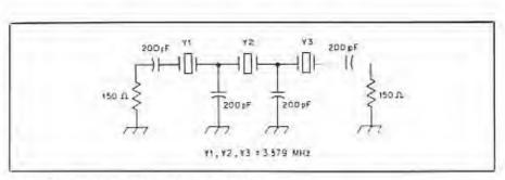
Fig 2-A simple CW filter using three crystals.
