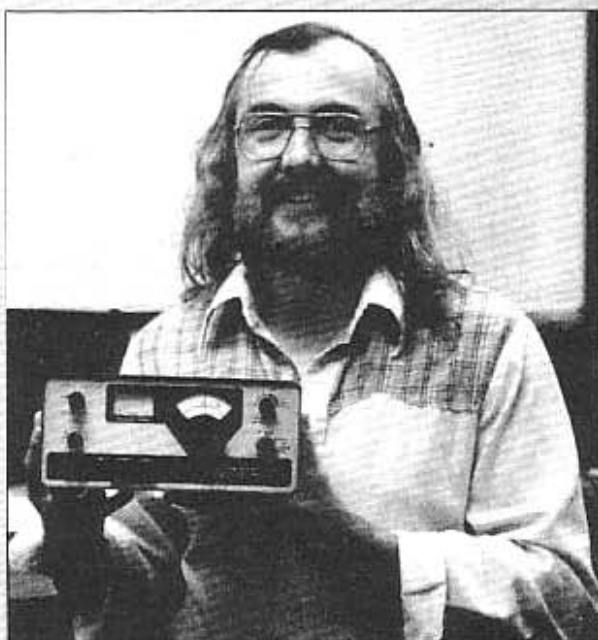
ARRL Lab Engineer Ed Hare, KA1CV, shows off his modified Heath HW-8 QRP transceiver. Ed's micro-power rig puts out slightly less than 10 milliwatts on 80 through 15 meters.
