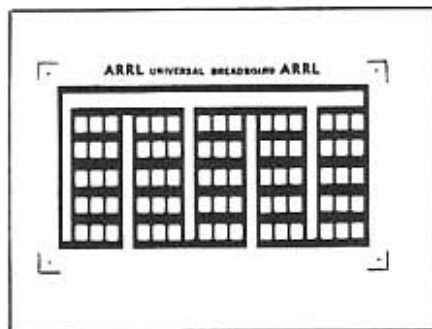
Fig. 5 — Suggested pattern for a universal breadboard that can be etched as shown, not to scale. A +V and a ground bus are provided for easy access along the length of the board. See the "Hints and Kinks" section of this issue for a full-size pattern template.
