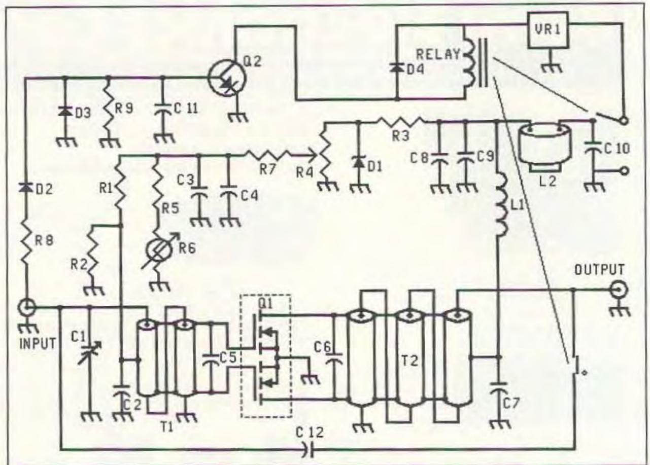
Figure 1. Schematic for the MRF175GV amplifier.
