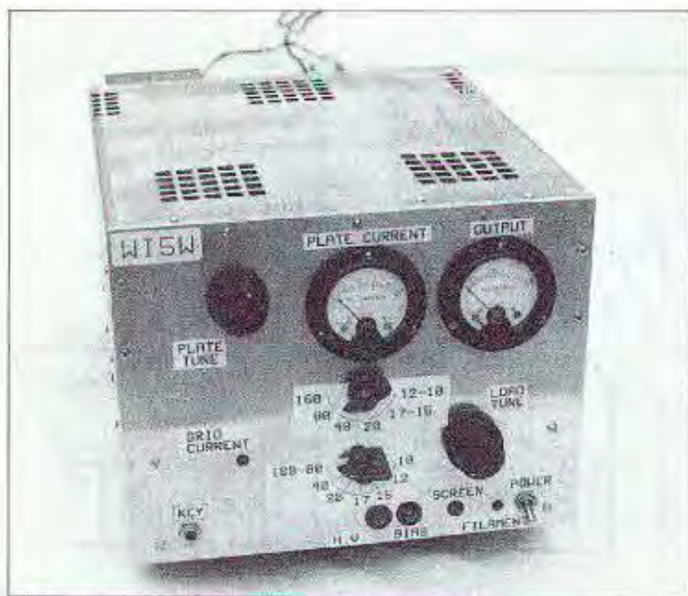
Photo A. The U-shaped top cover is salvaged aluminum and was formed using steel angle stock clamped to the work bench. The final angles of the corners were hammered into shape.
