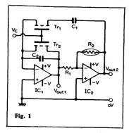
Typical performance Supplies  $\pm 15V$ IC<sub>1</sub>, IC<sub>2</sub> 741 Tr<sub>1</sub>, Tr<sub>2</sub>  $1/6 \times \text{CD4007AE}$ R<sub>1</sub>  $150\Omega$ R<sub>2</sub> thermistor type R13 C<sub>1</sub>, C<sub>2</sub> 100nF  $V_{\text{out}_1}$  520mV pk-pk  $V_{\text{out}_2}$  1.04V pk-pk See graph for f/V<sub>c</sub> (Fig. 2)
