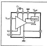
Typical data IC  $\frac{1}{2}$ SN74S124N C<sub>1</sub> 220pF  $V_s = V'_s + 5$ V d.c. Frequency range 0.7 to 1.8MHz (approx. linear)
