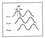
and maintaining as close a ratio as possible between the R values. Frequency is approximately 1/3RC. Note that with the CR values necessary for 60° phase shift at a specific frequency, the output of each buffer stage is attenuated by about one half and hence the minimum gain of each stage must be > 2.
