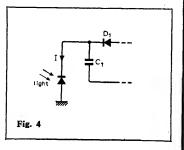
Most of the circuits described have been aimed at linearizing the v-f conversion, as in measurement of modulation systems. Sometimes it is required to have a converter in which the v-f conversion is highly non-linear with the frequency following, for example, an exponential or logarithmic function or sharply changing at some threshold voltage. The circuit indicates a simple way of changing the frequency over a claimed five-decade range.
