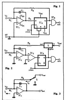
Typical performance of Fig. 1 IC<sub>1</sub> 741, IC<sub>2</sub> 1×CD4013AE IC<sub>3</sub> ½×CD4011AE Supplies  $V_{\rm DD}$  +10V  $V_{SS}$ -10V  $R_1$ ,  $R_2$  100k $\Omega$  $R_2 1k\Omega$ C<sub>1</sub> 100nF Clock 6V positive pulses, p.r.f. 1kHz, duty cycle 10% See Figs 4 and 5.
