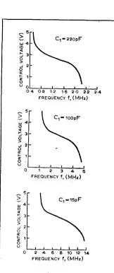
(no. 11) must be grounded for continuous output at the output terminal. Output is disabled if this terminal is taken to logic high or open-circuited. Graphs opposite indicate linearity over a restricted range for each capacitor value, and waveform deteriorates at very low values of C<sub>1</sub>, and thus at high frequencies.
