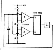
Fig. 12. Triangular wave generator using technique of Fig. 11.
