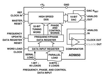
Figure 3. Block diagram of AD9850 125 MHz C-DDS.
