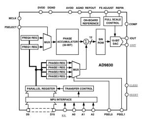
Figure 2. Block diagram of AD9830 50-MHz C-DDS.
