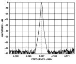
Figure 6. AD9830 narrowband spectral plot at 4.1 MHz Aout (50 MHz clock).
