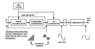
Figure 1. Basic Complete-DDS system block diagram.
