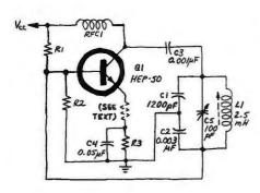
Fig. 4. Here we have added some values and a tuning capacitor.
