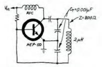
Fig. 3. Start with this basic Colpitts oscillator circuit.
