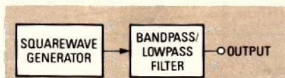
FIG. 7—LOWPASS OR BANDPASS FILTERS can clean up a squarewave source and provide a pure sine wave output.
