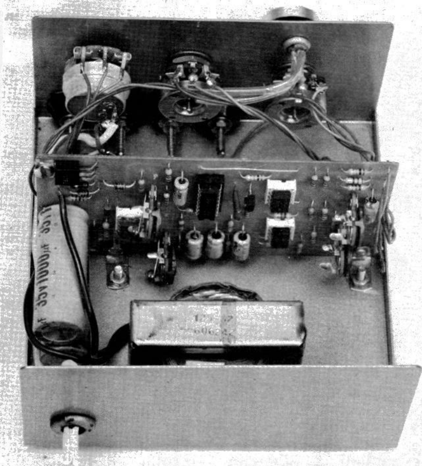
INTERIOR VIEW of fully-assembled unit showing details of point-to-point wiring. Angle brackets should contact bare metal in cabinet to assure good ground for shielding purposes. Binding posts are located just beneath front panel controls.
