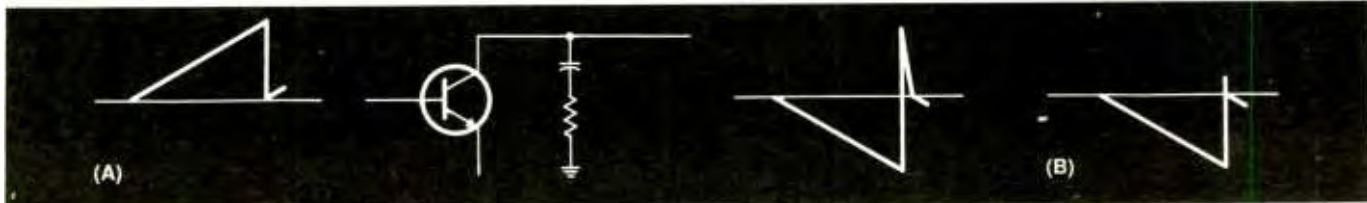
Fig. 7. Basic peaked-sawtooth wave-shaper (A) and low-amplitude peaking pulse (B) results from capacitor leakage.
