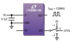
Figure 1. Fixed Frequency Silicon Oscillator
