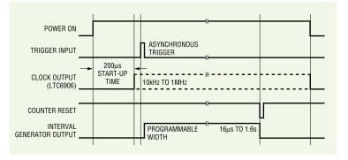
Figure 4. Timing Diagram for Time Interval Generator
