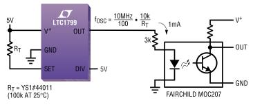
Figure 7. Remote Thermal Sensor Using a Thermistor
