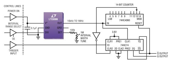
Figure 3. Micropower Tunable Time Interval Generator
