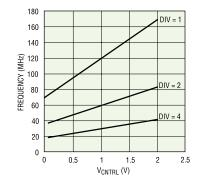
Figure 6. VCO Frequency vs. Voltage at Various Divider Settings
