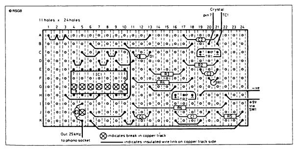
Figure 2 Stripboard, such as Veroboard, should be cut as shown to approx.  $62 \times 28$  mm
