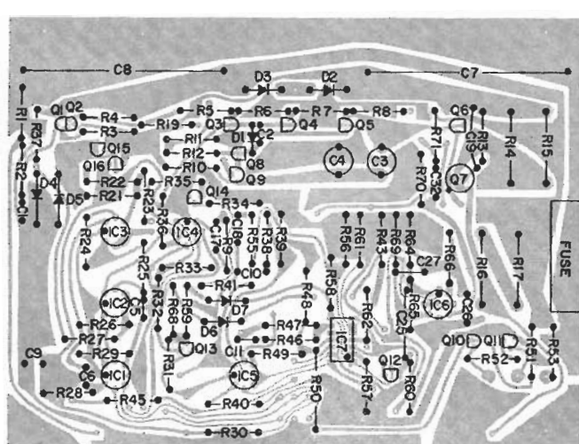
PRINTED-CIRCUIT BOARD DETAILS. Diagram at the top left shows the locations of jumper wires on the circuit board. The table at the left presents jumper details. Above is a diagram of parts positions on the circuit board. Follow it precisely. Below is the circuit board itself, as seen from the foil side. Actual size is 8-inches wide.
