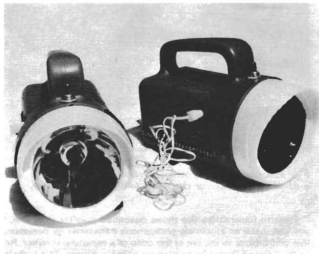
Fig. 5. Photophone receiver (left) and LED voice transmitter installed in 6-volt lantern lights. Note the position of the two back-to-back solar cells in the receiver's reflector.
