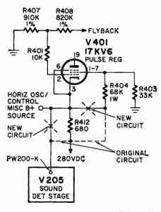
ure. Symptoms for R412 failure in sets with these changes are: no sound, no raster.—RCA Television Service Tips R-E
