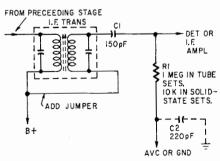
same time. You will need a 150-pF capacitor (C1) and either a 1-meg resistor for tube sets or a 10,000 ohm unit for the solid-state jobs (R1). In some cases, a 220-pF capacitor (C2) will be needed when the second i.f. is converted. The R1-C2 network takes
