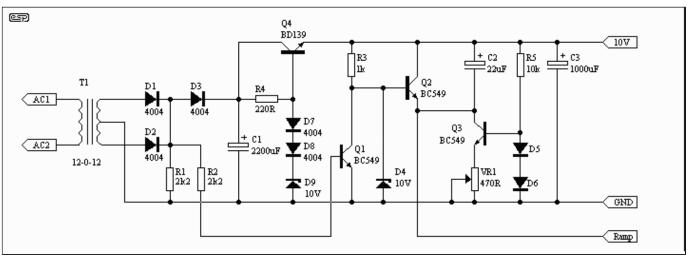
Figure 8a - New Ramp Generator Circuit
