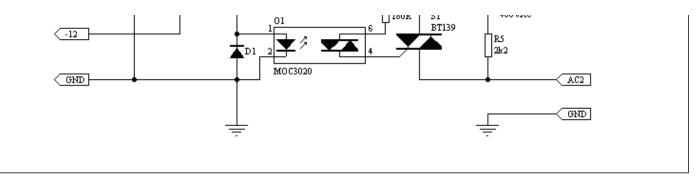
Figure 10 - Dimmer Circuit
