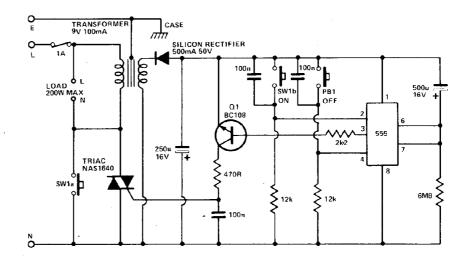
it must be rated accordingly. SW1b is used to trigger the 555 and start the timing period. Q1 will then be turned on, providing gate current to turn on the triac. When SW1 is released the supply and the load is maintained until the end of the timing period. PB1 is provided so
