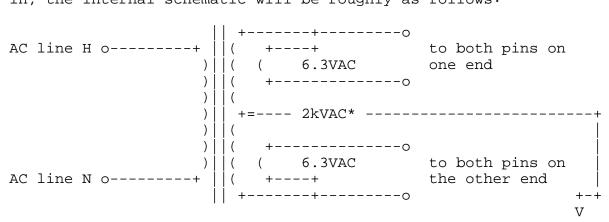
Most of the 48" 40-watt "shop light" type of bulbs use this. \*The high voltage winding of the secondary is on a branch magnetic circuit that limits the output current to the mercury discharge. Open circuit voltage will be in the kilovolt range, while the voltage across a lighted tube will be somewhat less than that and \_exceedingly\_ non-sinusoidal.
