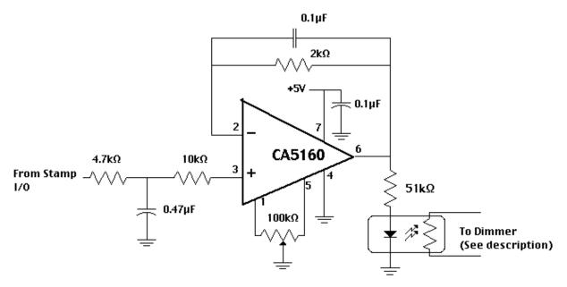
The circuit is simple, The op-amp provides current amplification allowing the optoisolator to sink current without discharging the  $4.7\mu F$  capacitor. The  $51k_{\rm m}$  resistor provides the right current through the optoisolator provide the right resistance on the output of the optoisolator.
