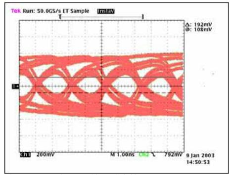
Figure 5a. Eye Diagram with 100ft Cables. 100ft, 480Mbps,  $t_{TJ}$ =660ps,  $t_{MJ}$  = N/A, 1.73 × 10<sup>13</sup> bits transmitted. No errors. Vertical scale: 200mV/Div. Horizontal scale: 1ns/Div.
