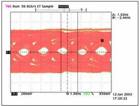
Figure 5b. Eye Diagram with 100ft Cables. 100ft, 520Mbps,  $t_{TJ}$ =1020ps,  $t_{MJ}$  = N/A, 1.87 × 10<sup>13</sup> bits transmitted. No errors. Vertical scale: 200mV/Div. Horizontal scale: 1ns/Div.
