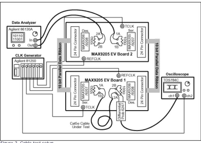
Figure 2. Cable test setup.
