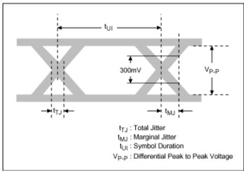
Figure 3. Jitter measurement definitions.
