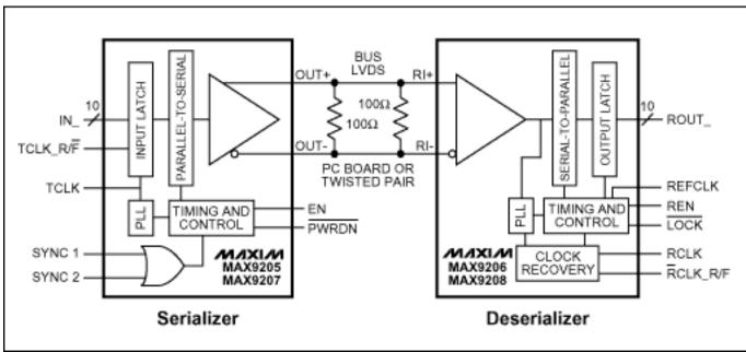
Figure 1. Serializer and deserializer functional block diagram.
