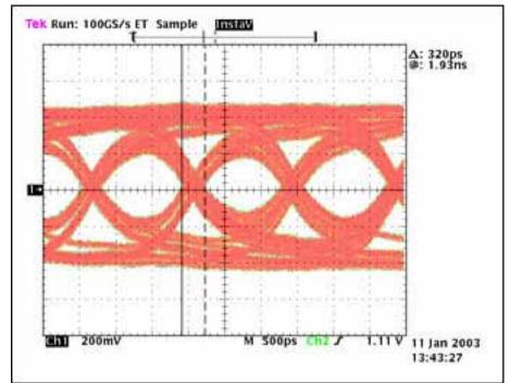
Figure 4b. MAX9207–MAX9208 Eye diagram with 60ft cables. 60ft, 720Mbps,  $t_{TJ}$ =320ps,  $t_{MJ}$  = N/A, 2.592 × 10<sup>12</sup> bits transmitted. No errors. Vertical scale: 200mV/Div. Horizontal scale: 500ps/Div.
