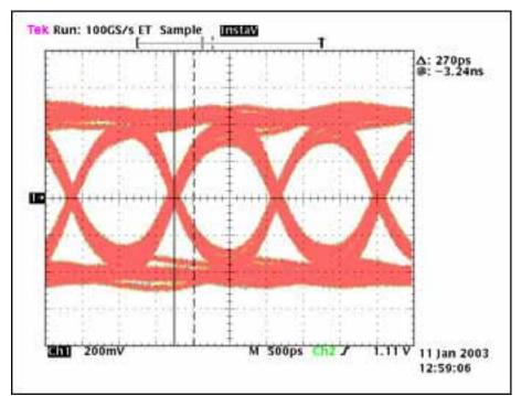
Figure 4a. MAX9207–MAX9208 Eye diagram with 30ft cables. 30ft, 720Mbps,  $t_{TJ}$ =220ps,  $t_{MJ}$  = 270ps, 2.592 × 10<sup>12</sup> bits transmitted. No errors. Vertical scale: 200mV/Div. Horizontal scale: 500ps/Div.
