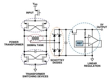
Figure 2. *iso*Power digital isolator implements isolated power.
