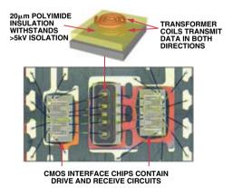
Figure 1. Construction of *i*Coupler digital isolator.
