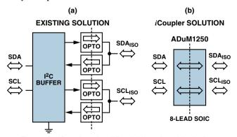
Figure 8. iCoupler simplifies bidirectional isolation.
