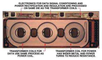
Figure 3. Chip-scale microtransformers.
