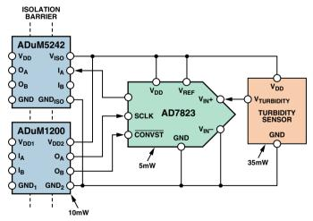
Figure 5. Isolated turbidity sensor.
