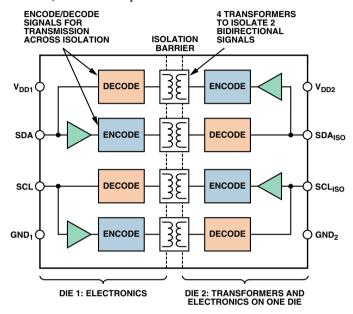
Figure 9. Bidirectional isolation using the ADuM1250.
