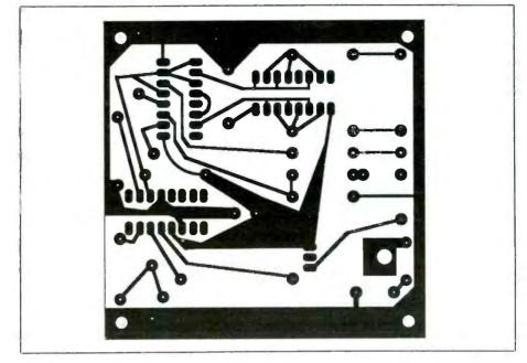
Fig. 3. Actual-size etching-and-drilling guide for project's printed-circuit board.
