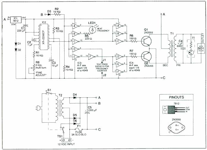
Fig. 2. Complete schematic diagram of Tide Clock electronic drive circuitry.
