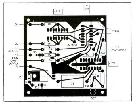
Fig. 4. Component-placement guide for pc board.
