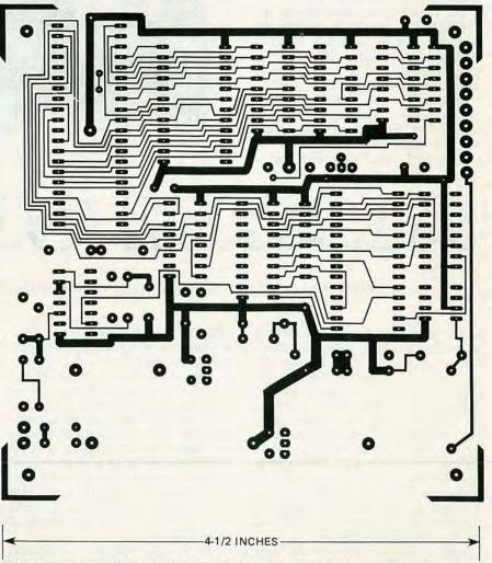
FIG. 5—COMPONENT SIDE of clock board. Large pads at right are for connections to switches and speakers.
