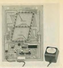
TOP VIEW of the PC board as it appears when the red plastic panel is removed. The six jumpers are clearly visible.
