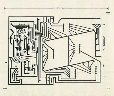
FIG. 2—PRINTED-CIRCUIT FOIL PATTERN is easy to duplicate photographically or by other means. An etched and drilled board is available at a moderate cost.
