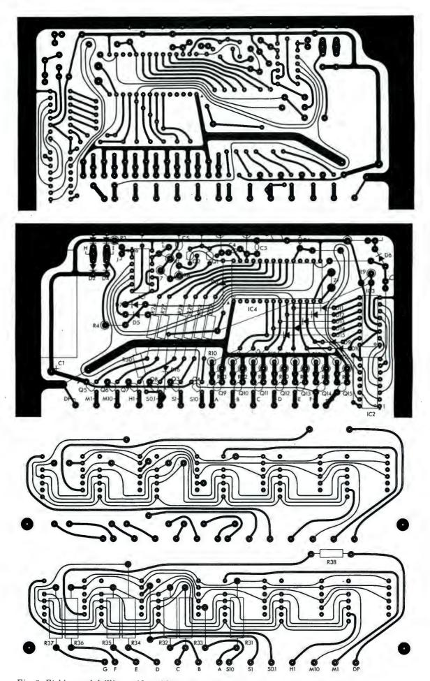
Fig. 2. Etching and drilling guides with component layout diagrams for the two pc boards.
