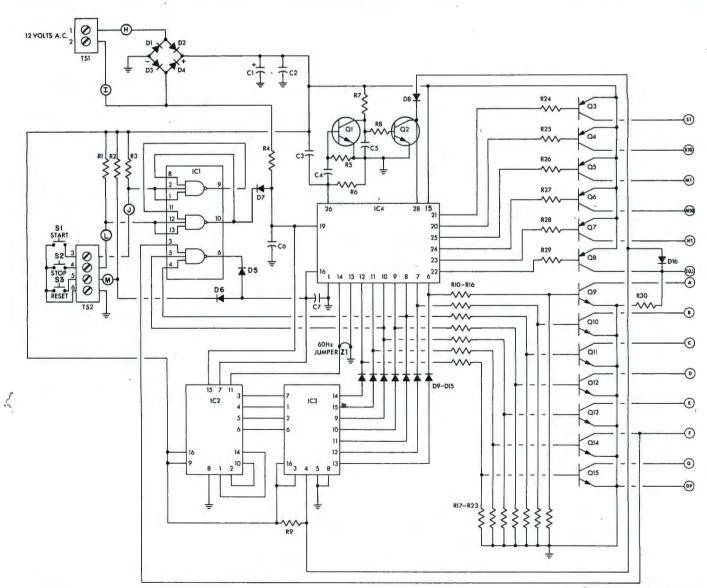
OULD you like to know precisely how long a recording session runs; how long it takes to make one lap around the track; or how long that new amplifier has been cooking on the bench? Here is a new six-digit stopclock that can do it-counting and displaying elapsed time up to ten hours by tenths of a second.
