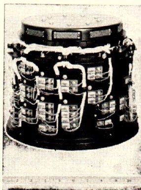
FIG. 14. TYPICAL MAGNETIC storage drum made by Computer Systems Laboratory of Litton Systems Inc. is for Litton's AIDE IV computer; capacity is 190,000 bits.
