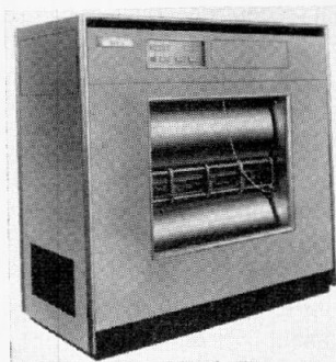
FIG. 18. REMINGTON RAND Randex twin-drum unit stores 24 million digits.
