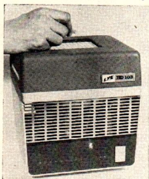
FIG. 12. LFE Model BD103 Bernoulli disc memory.
