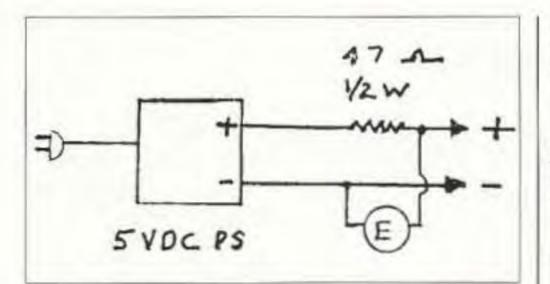
Fig. 5. A 5 VDC power supply, or a 3-6V battery, used for testing shorted components in the output circuits of a computer power supply.
