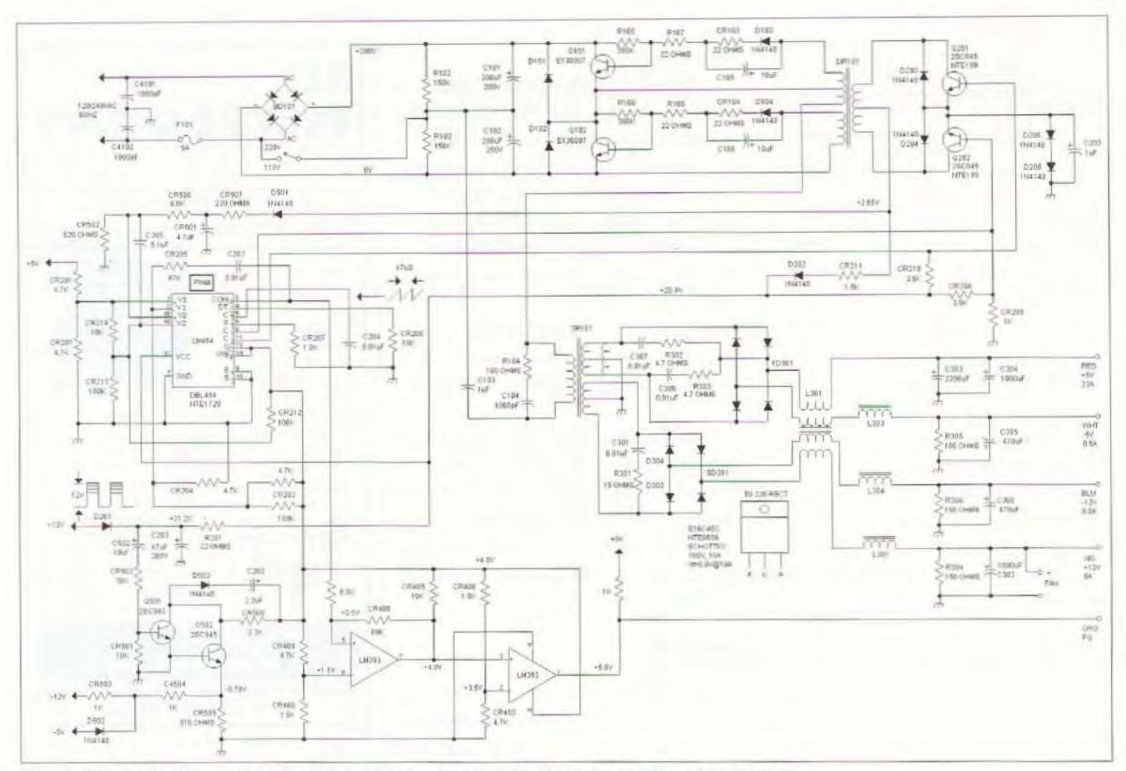
Fig. 7. Schematic of a typical non-ATX computer power supply that uses a voltage boost circuit.
