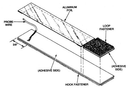
Fig. 4. Self-adesive Velcro-style hook-and-loop fasteners make assembly of the skin probes very simple. You could substitute a single layer of heavy-duty aluminum foil for the 2 layers of regular aluminum foil for the contact itself. With either type of foil, be sure to fold over the edges for added resistance to wear and tear on the probes.
