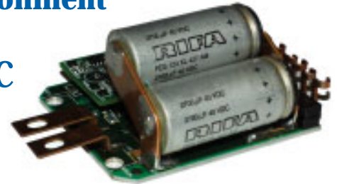
Electrolytic capacitors in an electric power steering controller.
