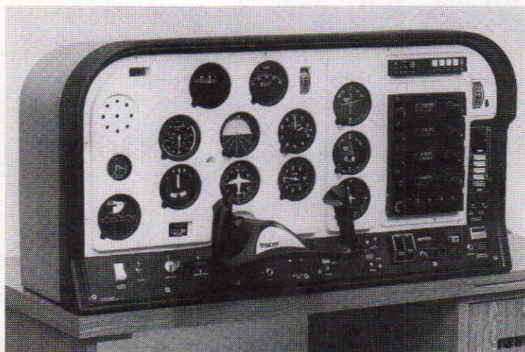
Fig. 12-8. Desk-top Pacer MKII flight simulator. (Courtesy Pacer Systems, Inc.)
