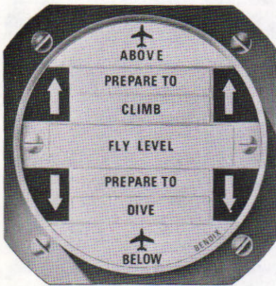
Fig. 1-15. The cockpit indicator of the Bendix collision avoidance system. (Courtesy Bendix Corp., Avionics Division)
