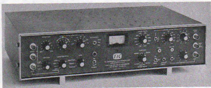
Fig. 8-17. The TIC Type T-16A DME Pulse Generator is a solid-state instrument that provides laboratory-quality impulses for DME checkout. (Courtesy Tel-Instrument Electronics Corp.)
