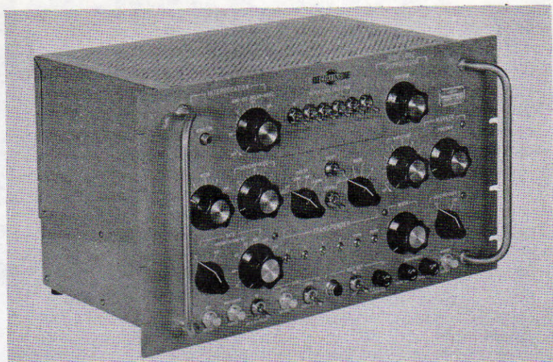
Fig. 9-18. The Collins 578X-1 ATC transponder bench test set. (Courtesy Collins Div., Rockwell International)
