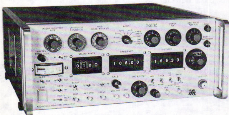
Fig. 8-19. The IFR, Inc., ATC-1200Y3 XPDR/DME Simulator may be used for both transponder and DME equipment. (Courtesy IFR, Inc.)
