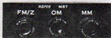
Fig. 6-9. Panel view of a NARCO MBT marker-beacon receiver. (Courtesy NARCO Avionics, a Division of NARCO Scientific Industries, Inc.)
