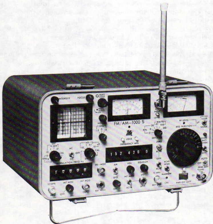
Fig. 3-22. The IFR, Inc., Model FM/AM-1000 S allows thorough check of a communication system from the ramp, or it may be used on the bench. (Courtesy IFR, Inc.)
