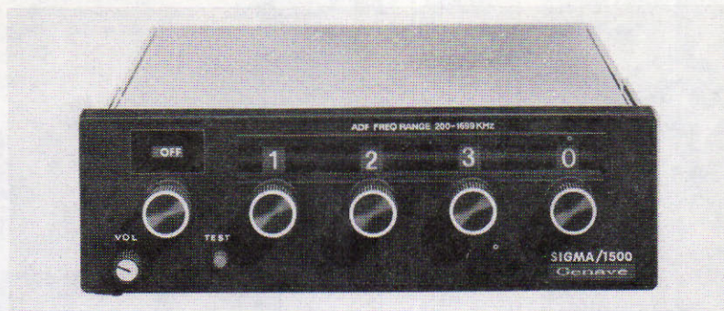
Fig. 7-17. The Genave SIGMA/1500 ADF uses PLL frequency synthesis to cover all 1-kHz increments from 200 kHz to 1699 kHz. (Courtesy General Aviation Electronics, Inc.)
