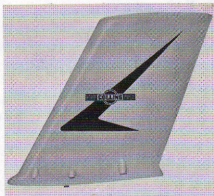
Fig. 2-11. A structure containing a vhf communications antenna designed for high-speed aircraft. (Courtesy Collins Div., Rockwell International)
