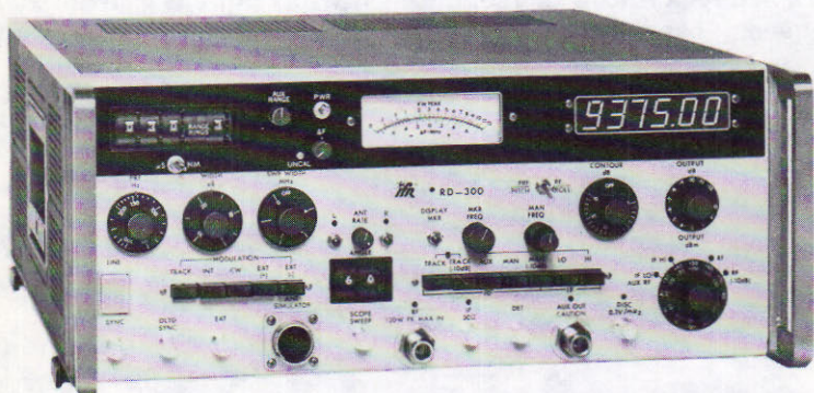
Fig. 10-11. The IFR, Inc., Model RD-300 weather radar test set. (Courtesy IFR, Inc.)
