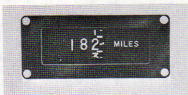
Fig. 8-1. Many DME systems provide an indication of distance on an instrument such as the one shown here.
