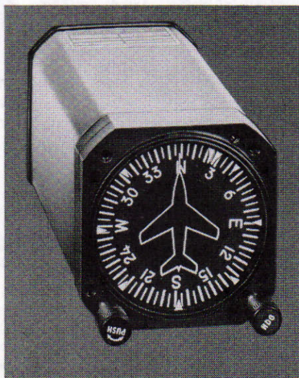
Fig. 13-6. The directional gyro of the Pathfinder is contained in this instrument. (Courtesy Astronautics Corp. of America)
