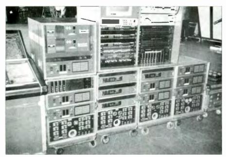
Figure 4. Power amps, equalizers, limiters, etc., used for the Alabama show.
